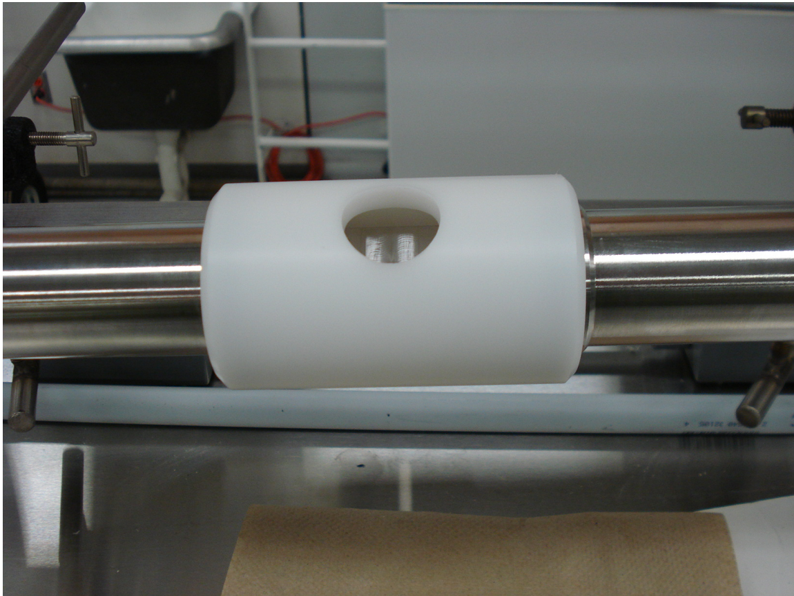
Figure 10: Offline measuring cell for Spectro::lyser™
