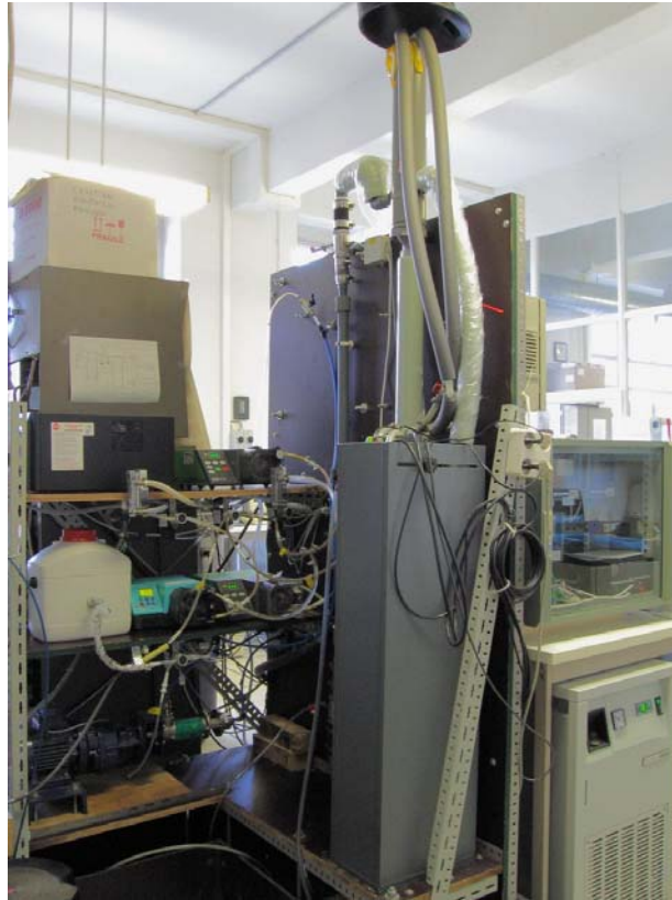
Figure 3-2 A view of lab-scale MBR system
