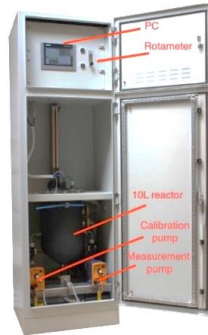
Figure 3-7 Schematic of RODTOX system
