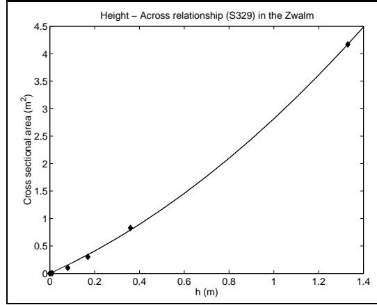
Figure 6.5: Calculated h - A_{cross} relationship for section 329
