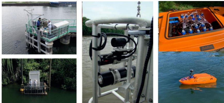
Figure 6: deployment of in-situ sensors and mobile sensors for real-time collection quality indicators. (© SIAAP Observatoire MeSeine [left and center], Fluidion DRONE [right] fluidion.com/en)
