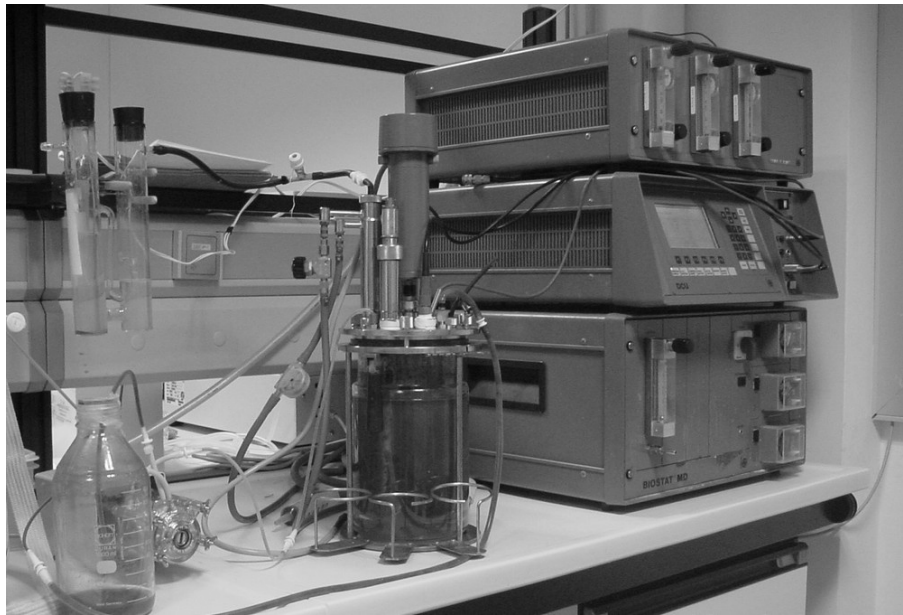
Figure 5.1 Experimental setup: transducers and data logging systems are to the right, the reactor, pH probe, gas flow sensor and gas sampling are in the middle and the thermal conductivity probe, influent /effluent pump and effluent sampling are to the left.
