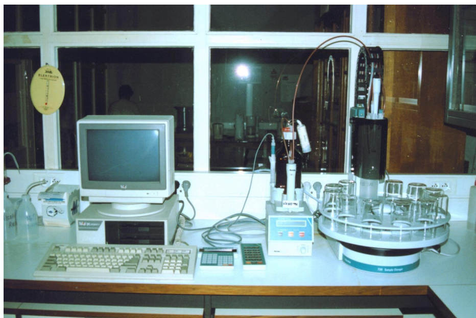
Figure 10.6 Experimental setup: PC on the left side, sample changer with samples in the glass pots on the right side, and Titrino 716 between PC and sample changer
