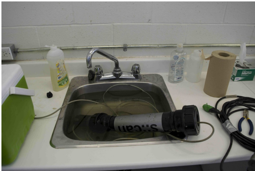
Figure 3: Cleaning of one of the sensor with water. Only water is allowed to use because other liquids could cause damage on the sensor.
