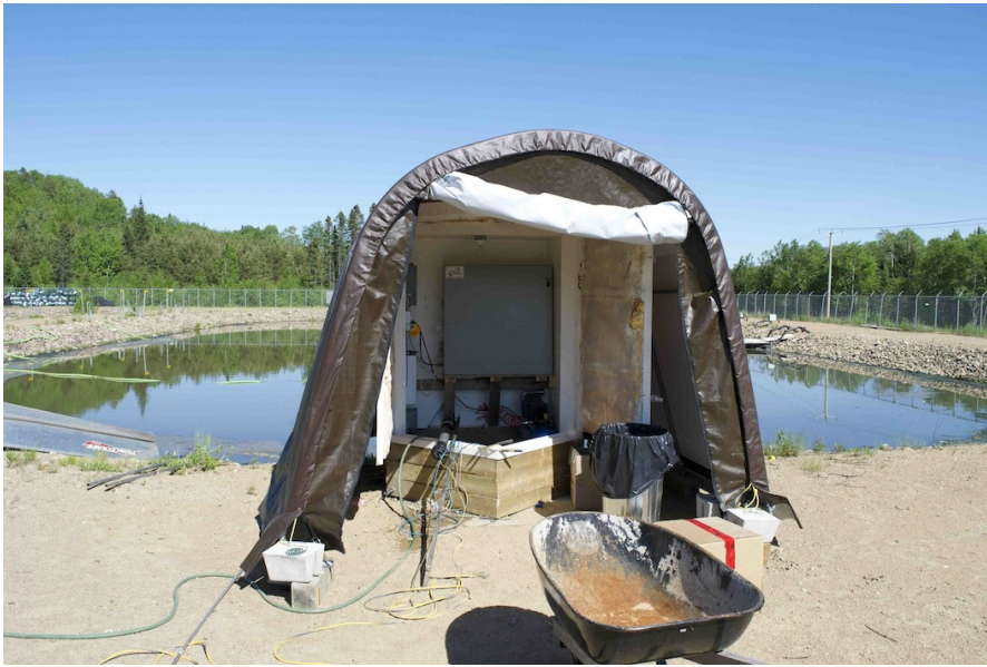
Figure 2: The first monEAU station at the inlet of the lagoon. The tent is for protection against wind and precipitation. The station is installed inside a big closet made out of solid metal and very thick isolation material to protect the system for freezing in the winter.
