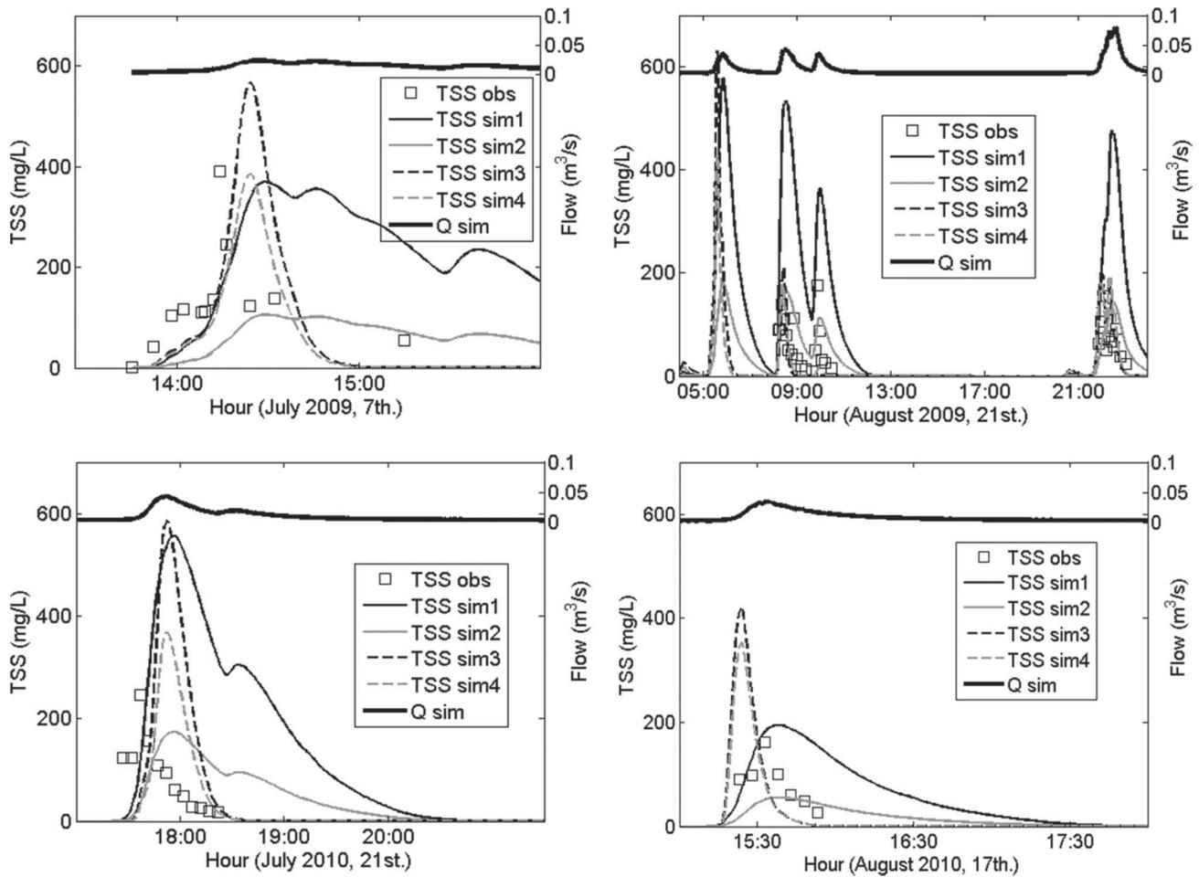
Figure 5. Observed (TSS obs) and simulated (TSS sim) TSS concentrations at the pond's inlet (validation period). The corresponding pond's inflow (Q sim) is represented on top of the graph. On the graph of the top right corner, TSS sim3 and TSS sim4 are merged for the main TSS concentration peak. See text for details.
