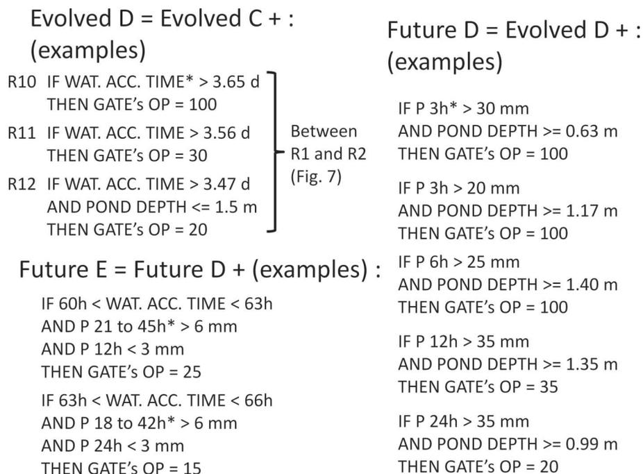
Figure 8. Rules of the “evolved D” strategy and examples of rules of the RTC scenarios relying in addition on forecast information; WAT. ACC. TIME = time spent with water accumulated in the pond (water accumulation time); P xxh = total rainfall depth forecasted over the next xx hours; Pxx to yyh = total rainfall depth forecasted between the next xx and yy hours.
