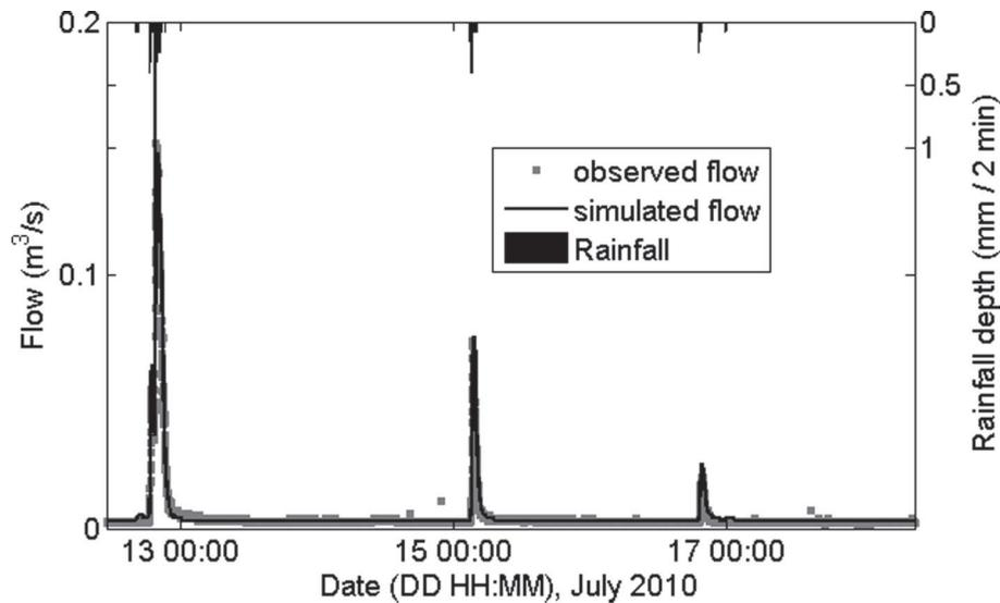
Figure 1. Observed and simulated pond's outflow with fully opened outlet (calibration period).
