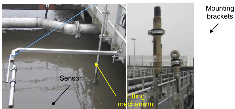
Figure 2. Details on sensors installation: Left: UV/Vis; Right: pH, conductivity.
