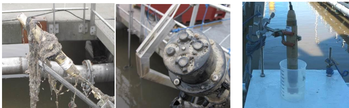
Figure 3. Maintenance routine: Clogging (left) and fouling (middle) of on-line water quality sensors, validation test of pH sensor (right).
