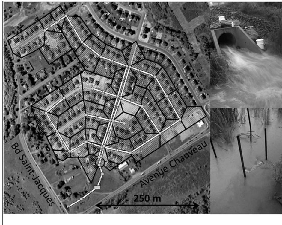
Figure 1. Map of the urban catchment discharging into the dry pond studied here (tank at the bottom of the image), and SWMM5 (see Section 2.2) schematic representation of the catchment's drainage network. The images in the top right and bottom right corners respectively show the inlet (outlet of the urban area) and outlet (dug between the posts) of the pond during a rain event.
