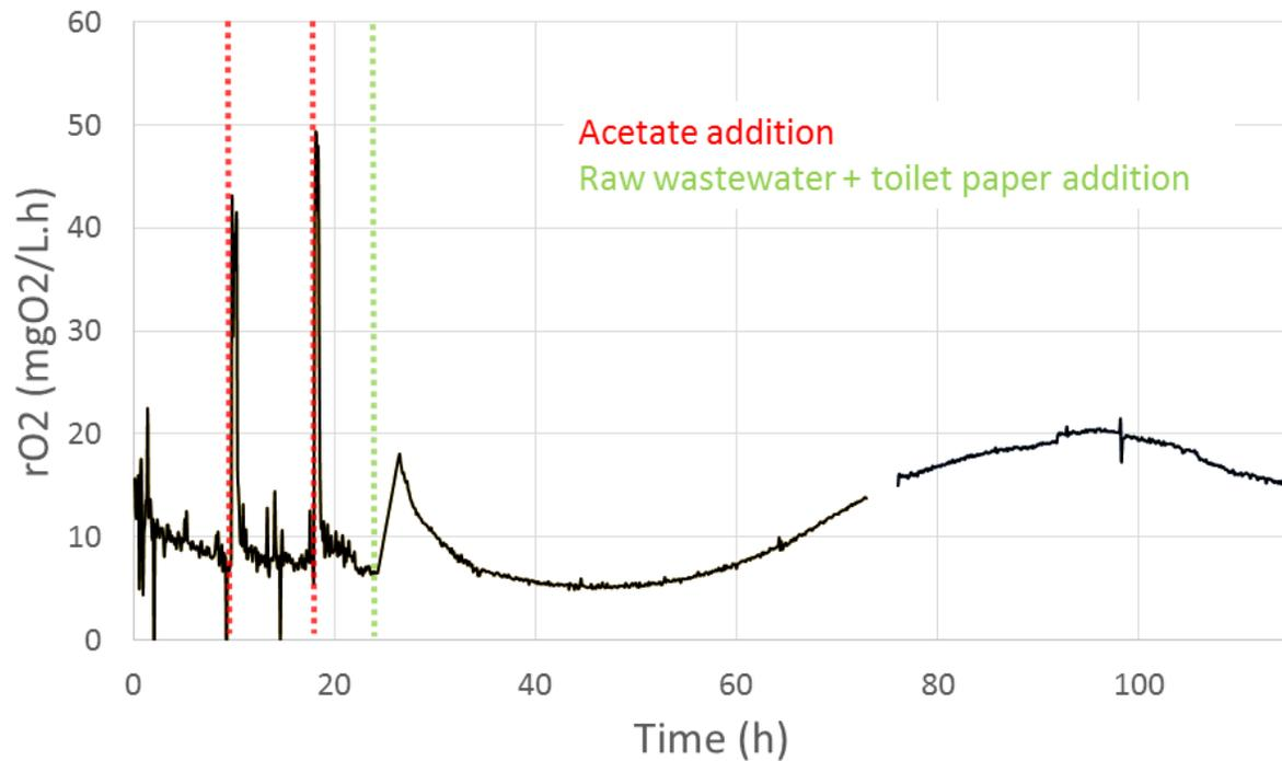
**Figure 3: Oxygen consumption rate in function of time measured in a respirometer with two additions of an acetate solution (at  $t=10\text{h}$  and  $t=18\text{h}$ , leading to initial concentration of  $78\text{ mgCOD/L}$ ) and an addition of raw WW spiked with  $5\text{g/l}$  of toilet paper (at  $t=24\text{h}$ , leading to initial concentration of  $5452\text{ mgCOD/L}$ ).**
