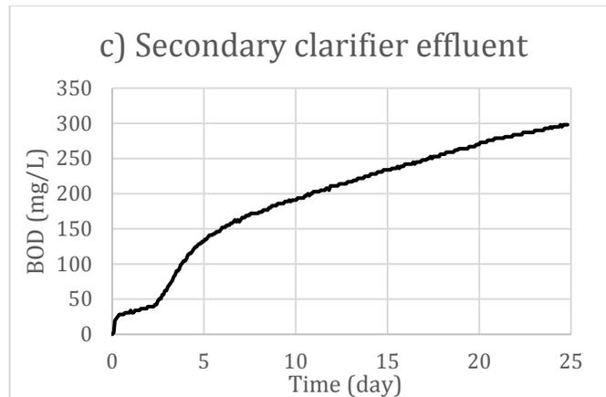
**Figure 4: BOD tests with toilet paper (5g/l) in different matrices**
