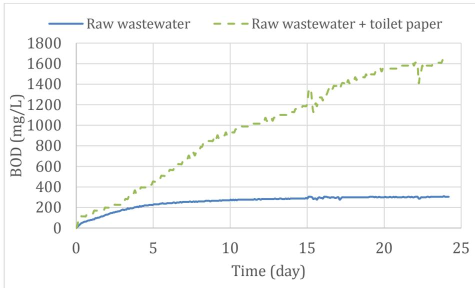
**Figure 1: Effect of addition of toilet paper on the BOD curve of raw wastewater**
