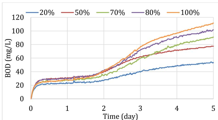
**Figure 5: BOD curves for toilet paper in different dilutions of secondary clarifier effluent. 20% signifies a mixture of 20% effluent and 80% tap water.**
