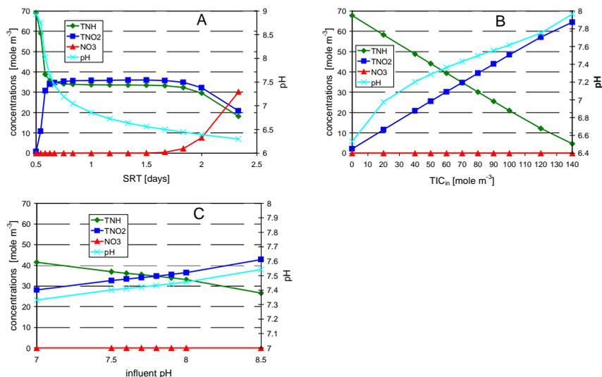
Figure 2 Influence of SRT (A), influent TIC concentration (B) and influent pH (C) on reactor concentrations and pH (steady state simulation results).
