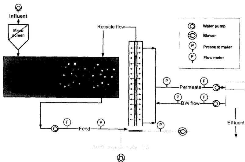
Fig. 1. Schematic of MBR pilot plant.
