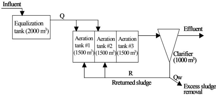
**Figure 1** Schematic diagram of cokes wastewater treatment plant
