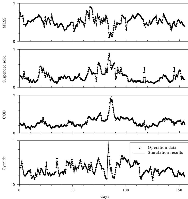
**Figure 4** Simulation results using the parallel hybrid model with NNPLS as non-parametric model
