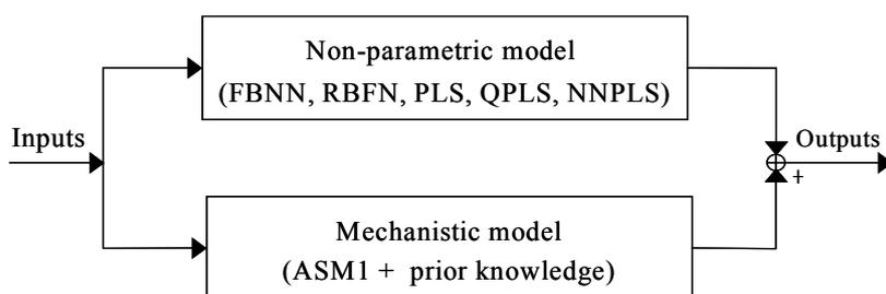
**Figure 2** Schematic diagram of the parallel hybrid model
