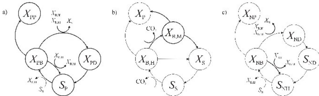
**Figure 1.** The fractionations and transformations of phosphorus (a), carbonaceous (b) and nitrogenous (c) state variables in the extended model. Notations are according to Henze *et al.* (2000) where not else notified. State variables and transformation arrows given in bold denote extensions that have been made to ASM1. Inert components originating from influents are not shown.
