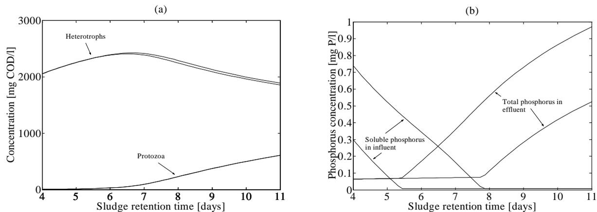
**Figure 2.** Steady-state solutions for simulations with different SRTs. Continuous lines: All phosphorus biodegradable. Dotted lines: 80% of particulate phosphorus biodegradable.
