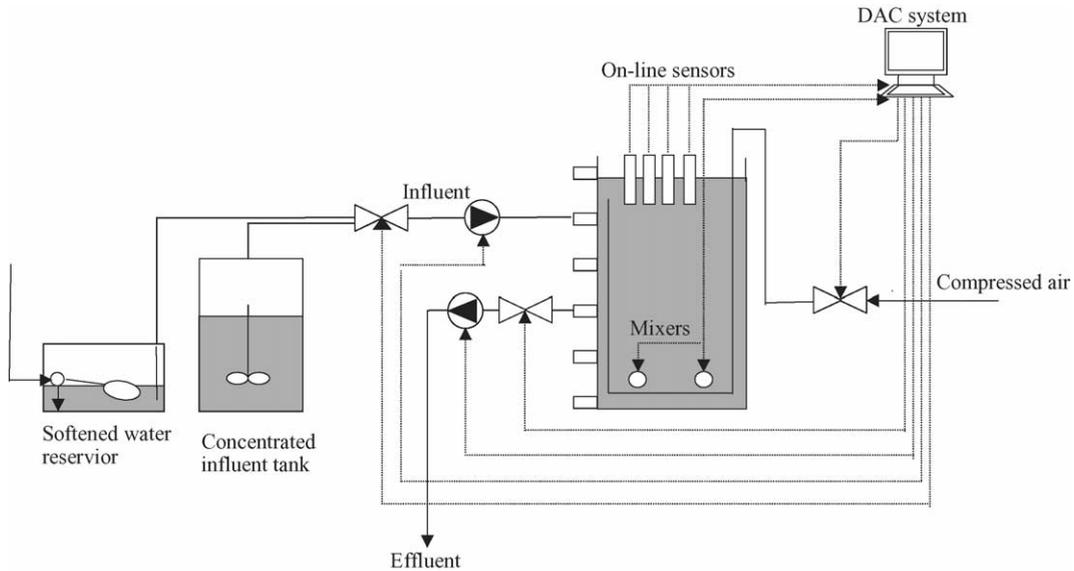
Fig. 5. Schematic diagram of a sequencing batch reactor system.
