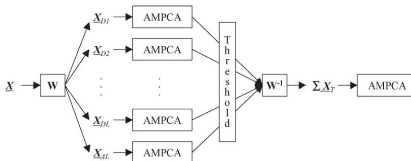
Fig. 4. Adaptive multiscale PCA (AMPCA) methodology.
