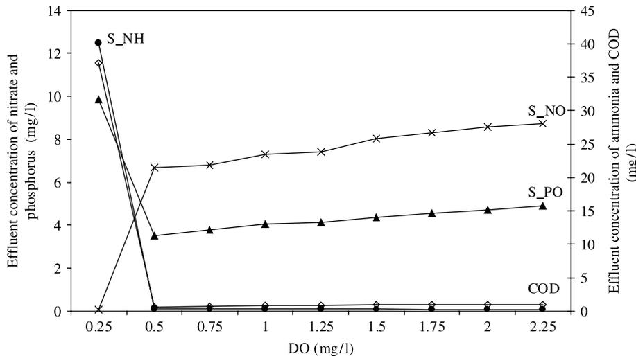
**Figure 4** Effluent phosphorus, nitrate, ammonia and COD concentrations for level 1 scenario analysis with varying DOsp (SRT = 17.5d and Qint = 0.864m³/d)
