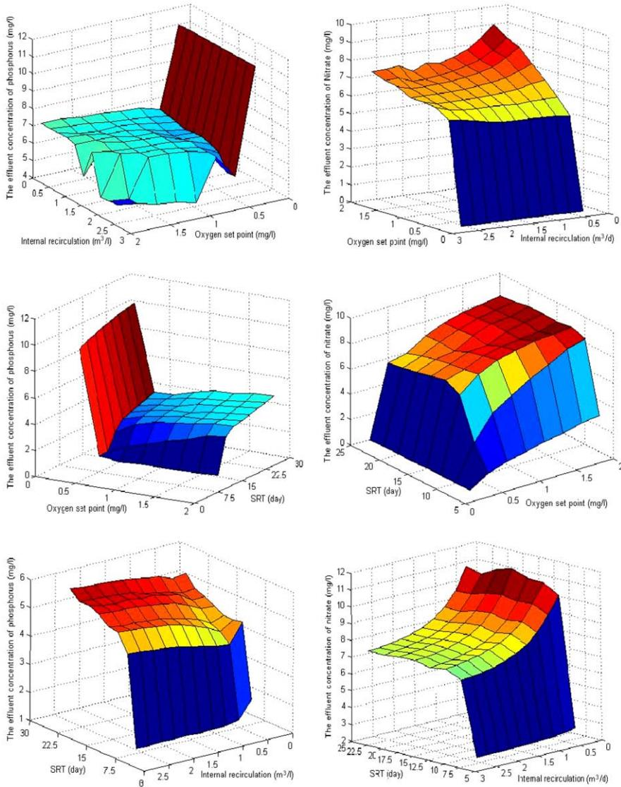
**Figure 6** Effluent phosphorous (left) and nitrate (right) concentration for the second level scenario analysis: fixed SRT (top), fixed Qint (middle), fixed DOsp (bottom)
