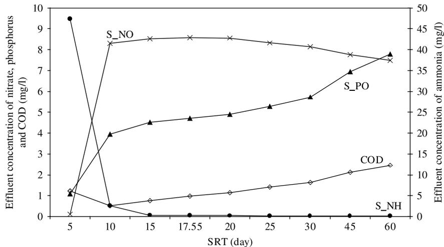
**Figure 5** Effluent phosphorus, nitrate, ammonia and COD concentrations for level 1 scenario analysis with varying SRT (DO = 2 mg/l and  $Q_{int} = 0.864\text{m}^3/\text{d}$ )
