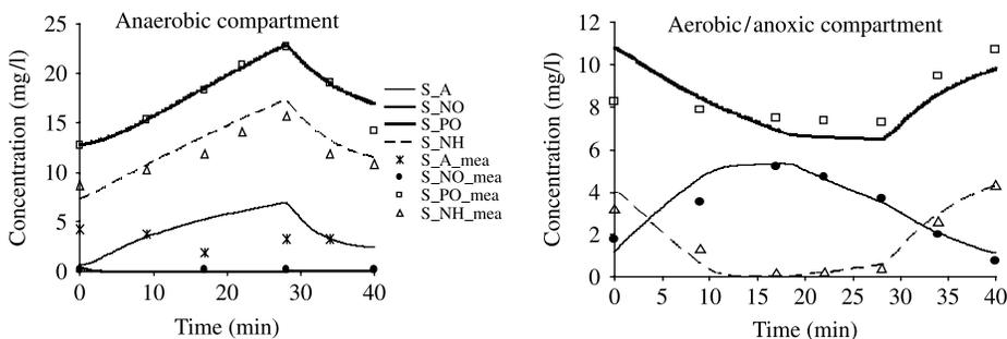
**Figure 2** Results of the calibration with the comparison of the simulation and measurements in the anaerobic and aerobic/anoxic compartment during 1 cycle ([Jiang et al., 2007](#))
