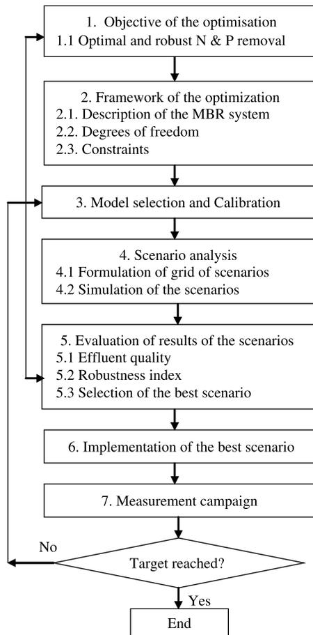
**Figure 1** A systematic methodology for the model-based optimisation of MBR systems (after Sin *et al.*, 2004)
