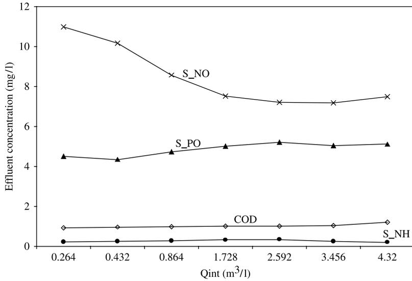
**Figure 3** Effluent phosphorus, nitrate, ammonia and COD concentrations for level 1 scenario analysis with varying Qint (SRT = 17.5d and DOsp = 2 mg/l)
