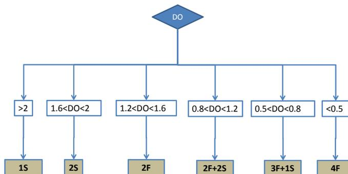
Figure 2. Decision tree for strategy 1 based on DO (mg·L<sup>-1</sup>) values (F: engine at fast speed, S: engine at slow speed).
