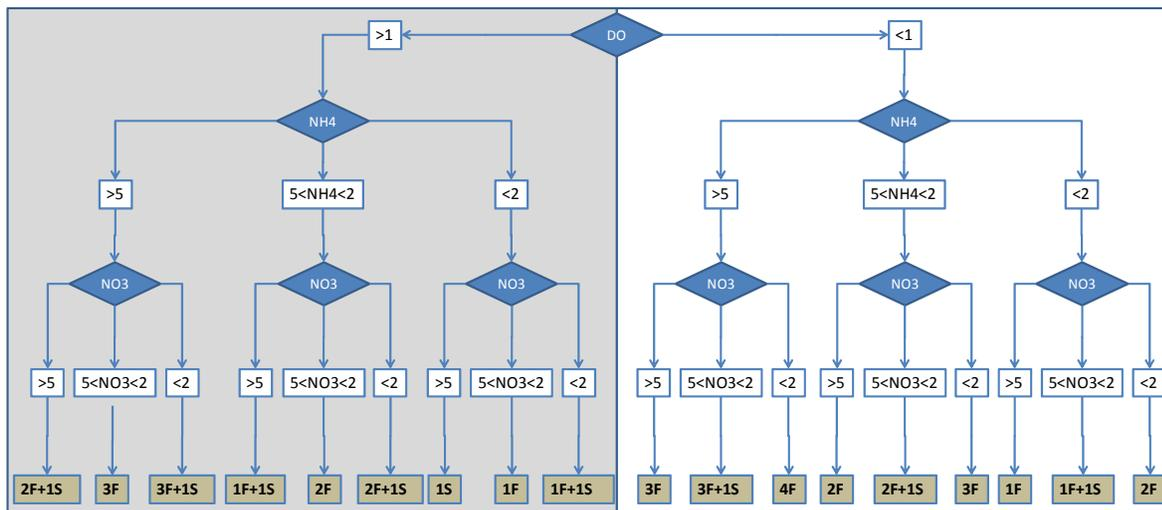
Figure 3. Decision tree for strategies 2 and 3 based on DO, NH<sub>4</sub><sup>+</sup> and NO<sub>3</sub><sup>-</sup> (mg·L<sup>-1</sup>) (F: engine at fast speed, S: engine at slow speed).
