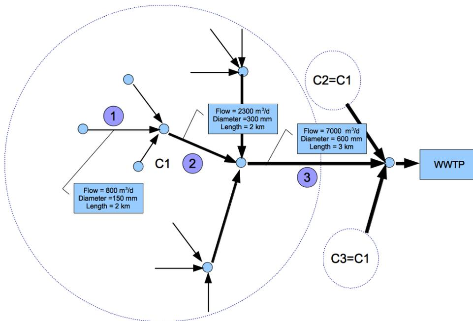
Figure 2 - Modelled Sewer Network
