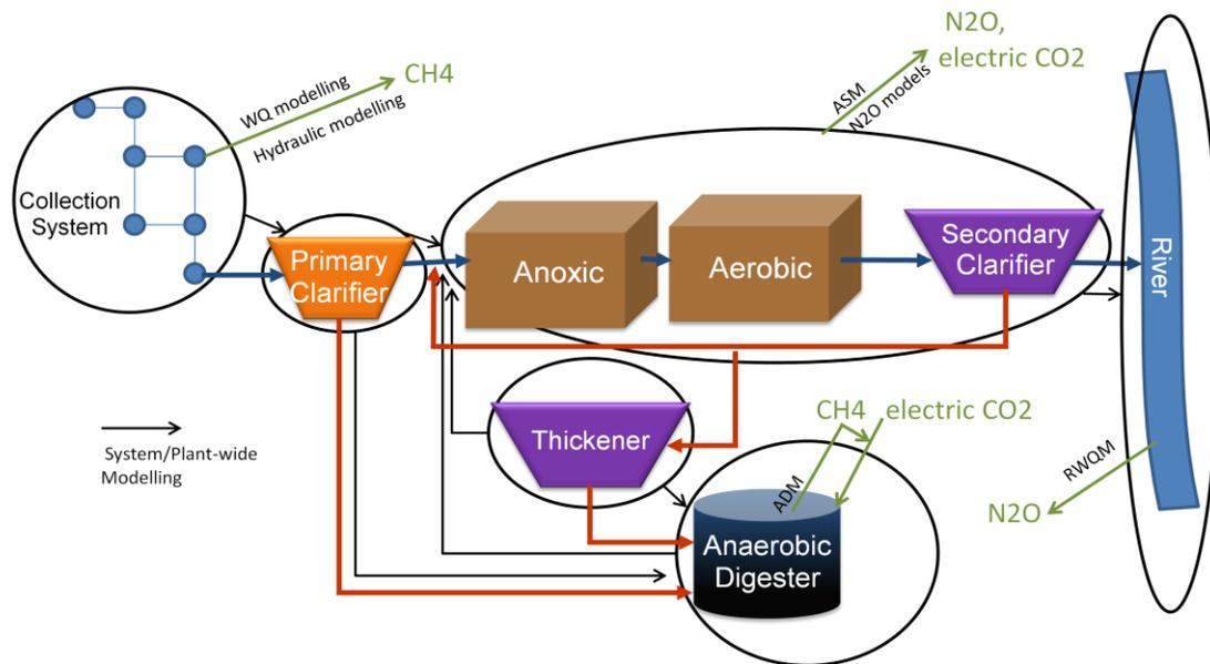
Figure 1 - System/Plant-wide GHG Modelling Schematic
