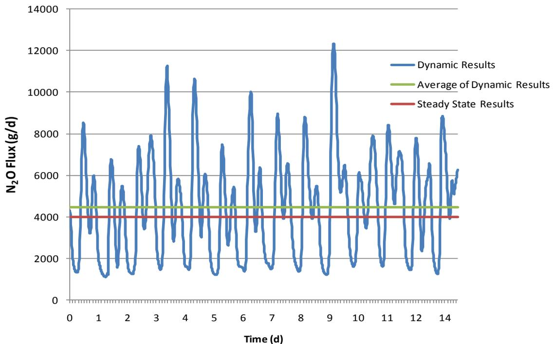
**Figure 6 - Steady State versus Dynamic Results for N<sub>2</sub>O flux in ASU3 (first aerobic reactor)**
