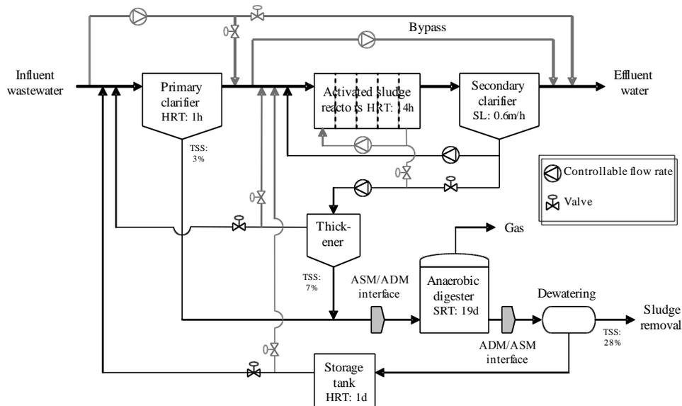
Figure 3 – BSM2 Plant Configuration (Nopens et al., 2010)
