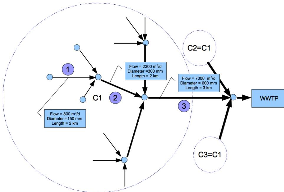
Figure 2 - Modelled Sewer Network
