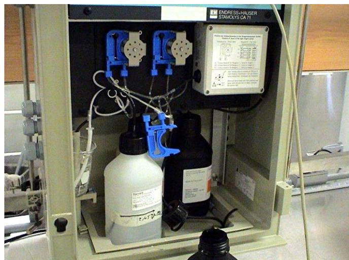
**Figure 16:** Simulation of a clogged reagent PH-A1 tube (similar buildup for reagent PH-A2)
