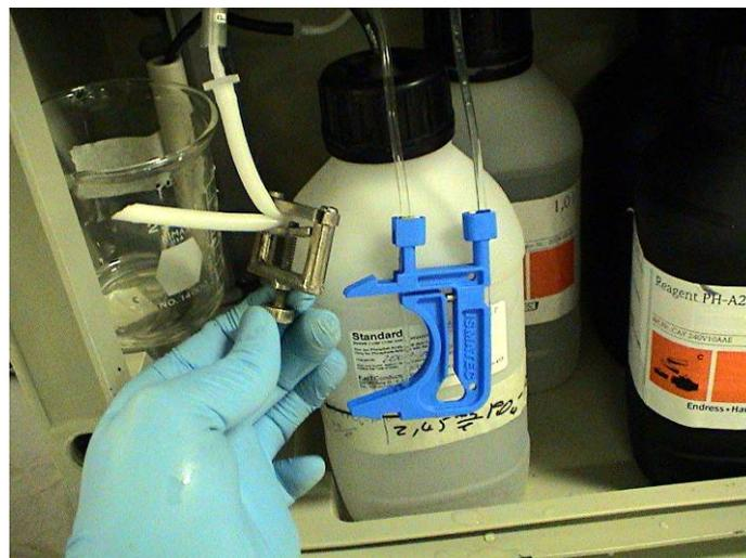
**Figure 12:** Pinched-off sample tube for experimental series
