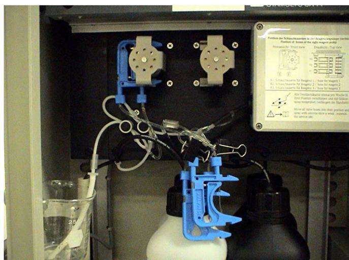
**Figure 14:** Simulation of reagent pump failure
