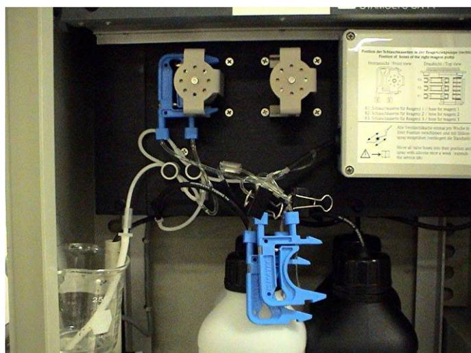
**Figure 14:** Simulation of reagent pump failure
