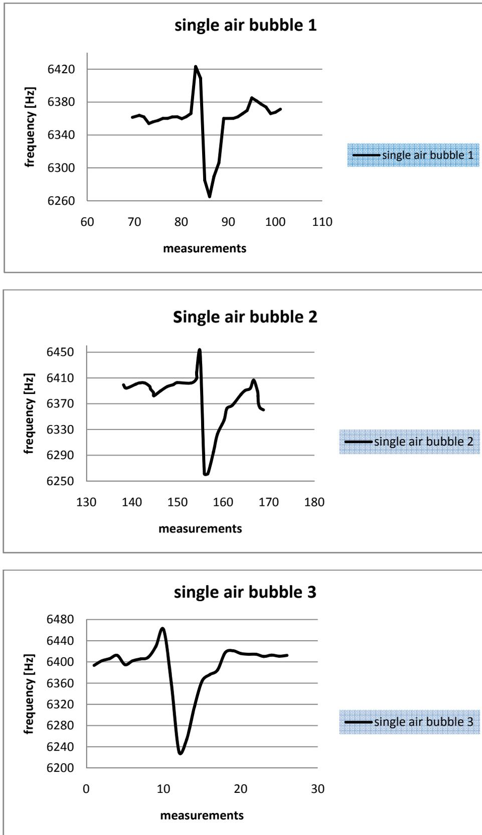
Figure 20: Typical pattern in the frequency curve, caused by air bubbles
