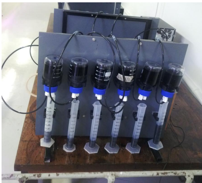
Figure 62: NaOH solution displacement
