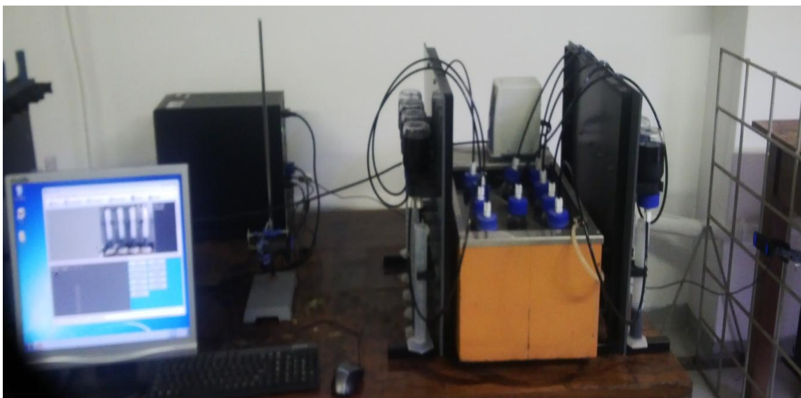
Figure 61: Serum Bottle setup including webcams for gas production observation
