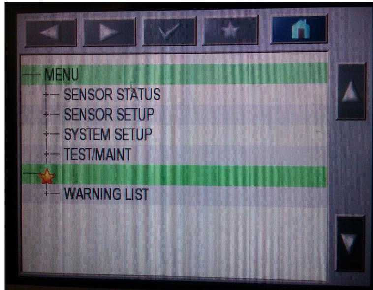
Figure 3.9: Main menu display of controller sc1000.
