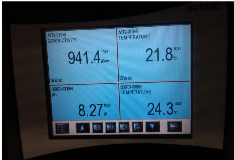
Figure 3.8: Interface and colour touch-screen display of controller sc1000.
