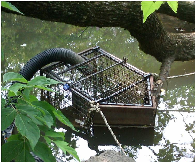
Figure 3.7: Installed sensors in the protective cage.
