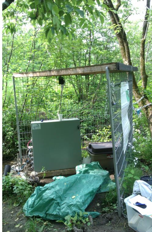
Figure 3.2: Installed RSM30 in protective cage.
