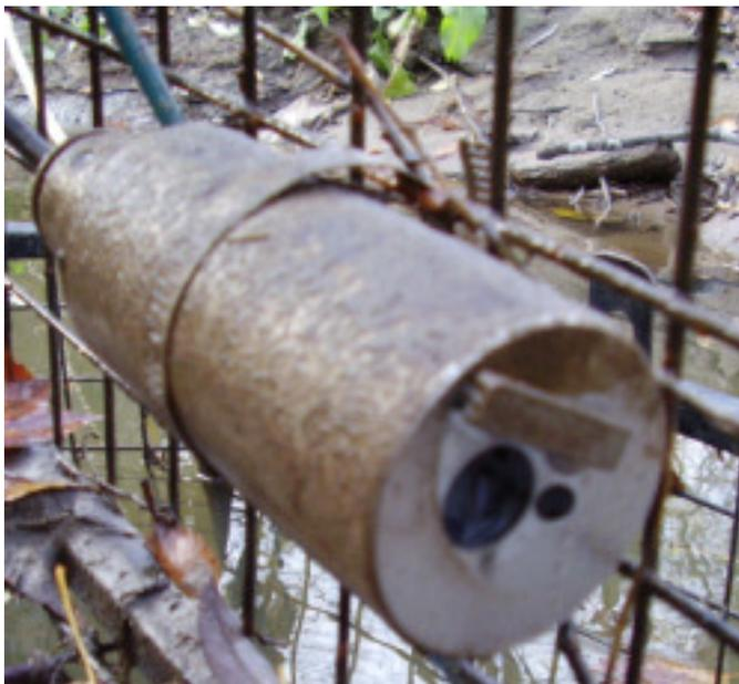
Figure 68 : Turbidity sensor with wiper
