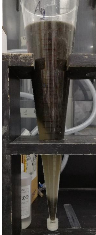
Figure 26: Primary sludge after 30 minutes of sedimentation in an Imhoff cone.
