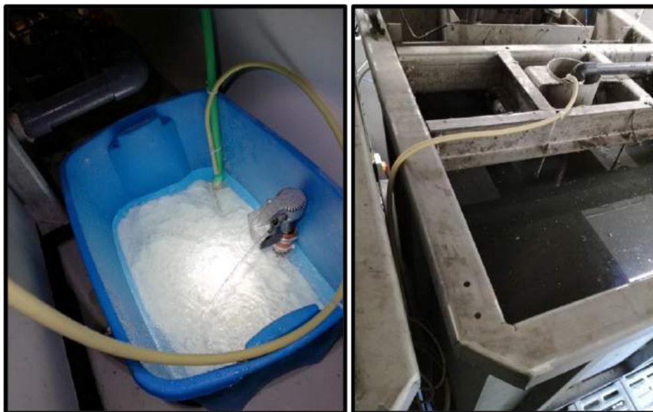
Figure A.2: Alkalinity dosage into the pilEAUte PST
