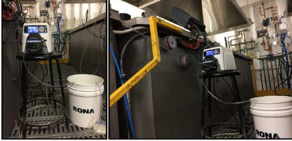
Figure A.1: Substrate dosage into the pilEAUte SST
