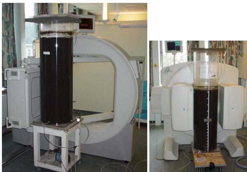
**Figure 5.3:** Experimental C-set-up at the Ghent University Hospital (left: lower section, 1500XP camera; right: upper section, AXIS camera)
