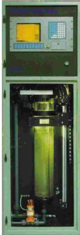
**Figure 7.3:** The Settrometer (Applitek N.V.; Vanrolleghem *et al.* (1996))
