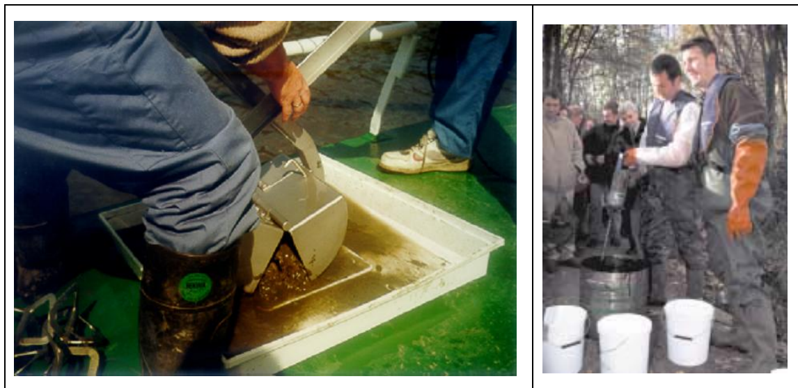
Figure 4.2 Van Veen grab sampler (left) and mixing to obtain homogeneous subsamples for the different analyses (right).
