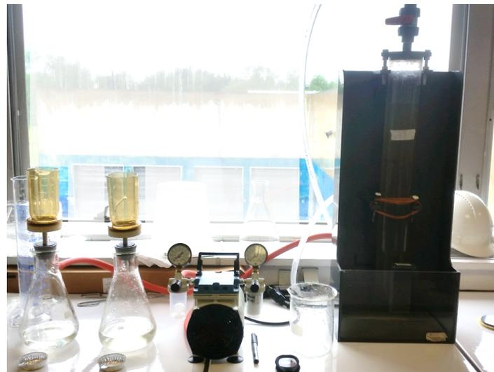
Figure 1.9: ViCAs experimental set-up as installed at the WRRF CdH with the settling column on the right-hand side.
