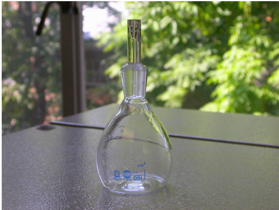
Figure 3.4: Illustration of a pycnometer
