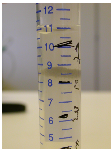
Figure 3.6: Real sample of a floc density measurement based on a Percoll density gradient ranging from 1.01 to 1.05 g.ml -1
