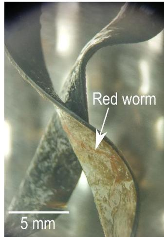
Figure 9.12: Colonized biofilm support media with presence of red worms
