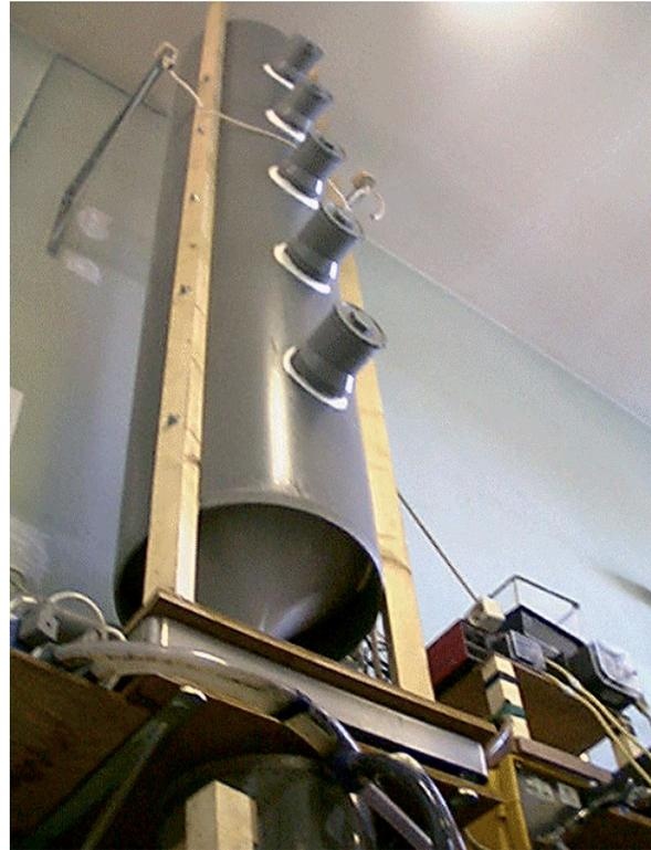
Figure 5.3: Scheme and picture of filter body
