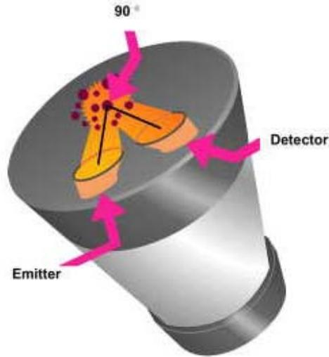
**Figure 1: turbidity sensor principle**
