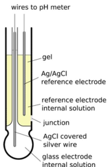
Figure 22: pH electrode explanation
