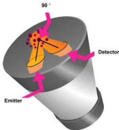
**Figure 20: Turbidity sensor principle**
