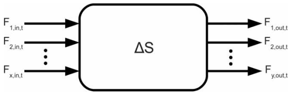
Figure 1 | Simple balancing layout. Several fluxes may enter or leave a system, accumulation ( \Delta S ) is possible.
