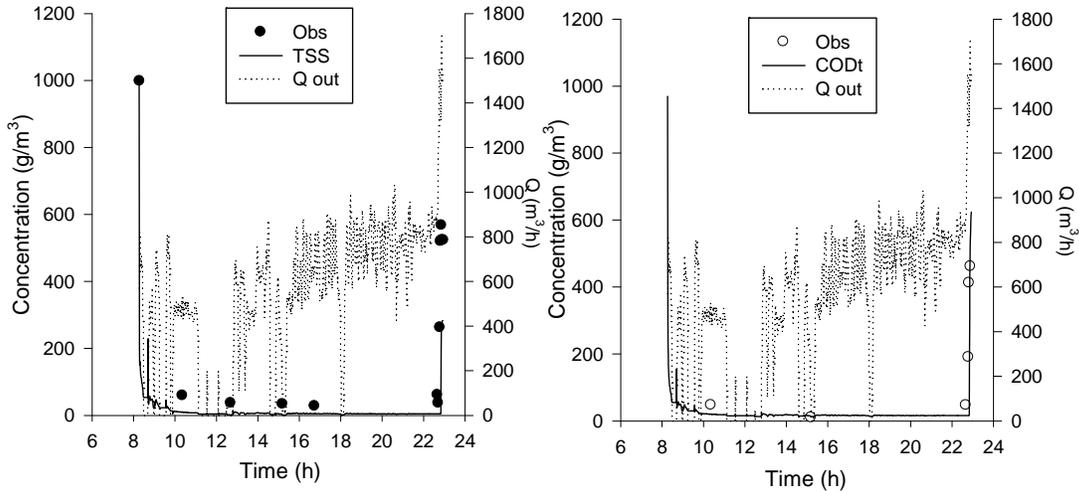
**Figure 7.** Calibration results for the September 27<sup>th</sup> 2009 event. a) On the left, the effluent TSS concentration; and b) on the right, the effluent CODt concentration.
