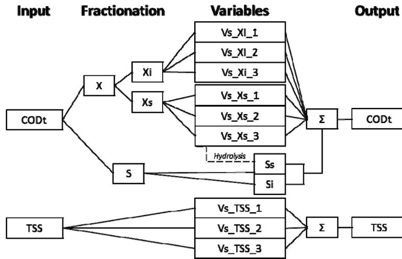
**Figure 1.** Fractionation concept of the collected data (*input*) to the model variables. Variables named “Vs\_XXX\_1,2,3” are subject to sedimentation/resuspension. Hydrolysis reactions occur between “Vs\_Xs\_1,2,3” and “Ss” variables.
