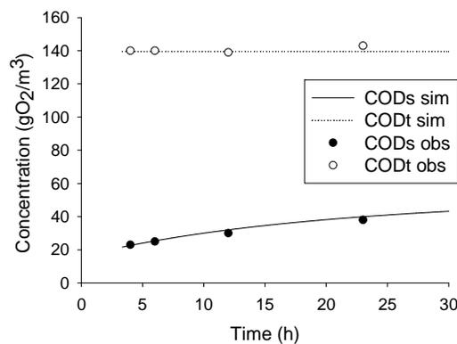
**Figure 5.** Calibration results of the hydrolysis rate.
