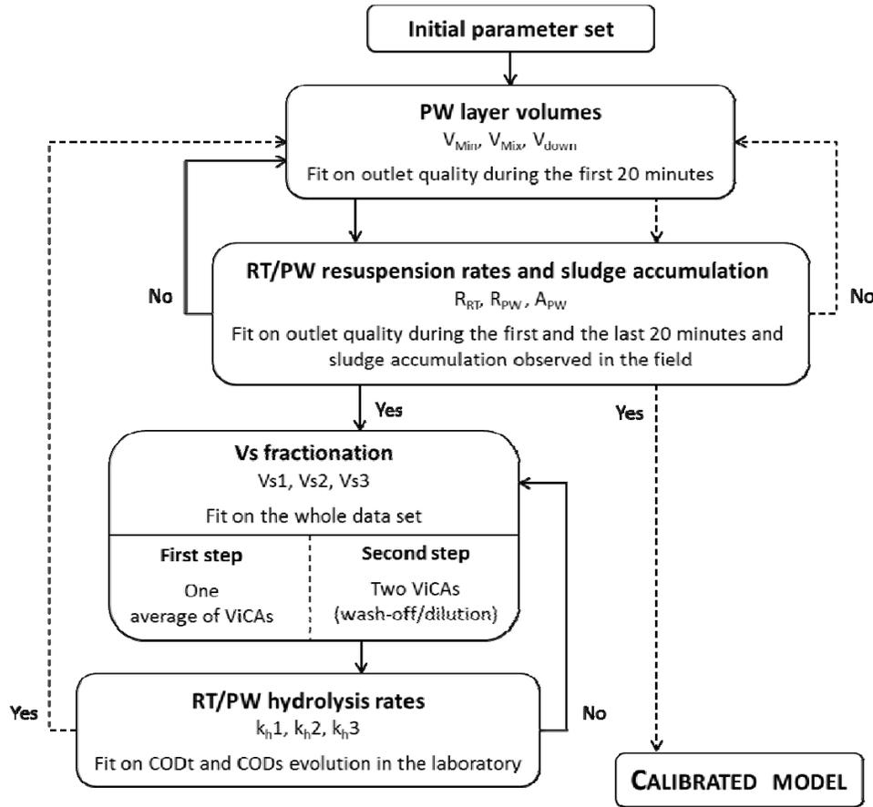
**Figure 3.** Model parameter calibration steps.
