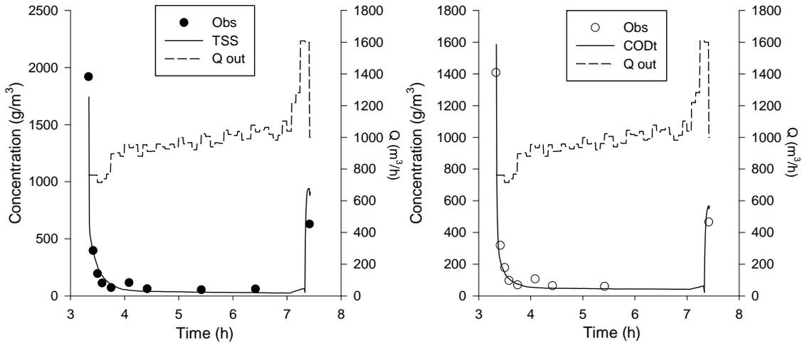
**Figure 6.** Calibration results for the July 27<sup>th</sup> 2009 event. a) On the left, the effluent TSS concentration; and b) on the right, the effluent CODt concentration.
