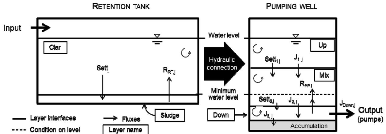
**Figure 2.** RT/PW model conceptual diagram from Maruejous *et al.* (2012) improved by three ways.
