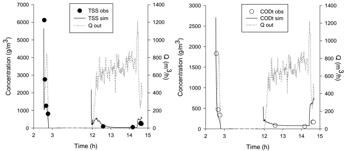
**Figure 8.** Validation results for the July 13<sup>th</sup> 2010 event. a) On the left, TSS effluent concentrations; and b) on the right, CODt concentrations.
