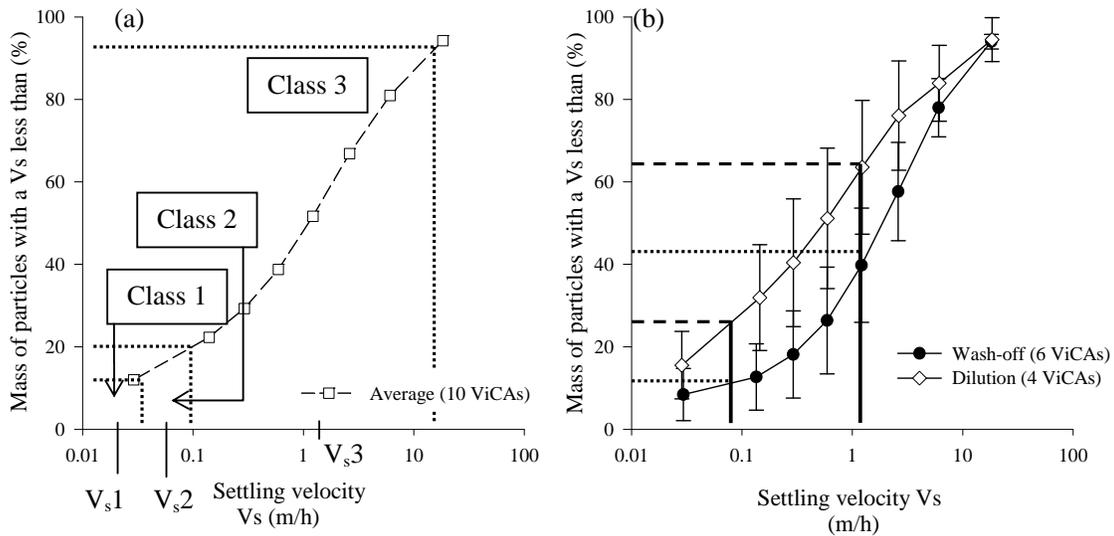
**Figure 4.** Vs fractionation description for the three classes' definition. a) Calibration on one ViCAs average; and b) Vs distributions used for calibration on two ViCAs averages ("Wash-off" and "Dilution" periods).
