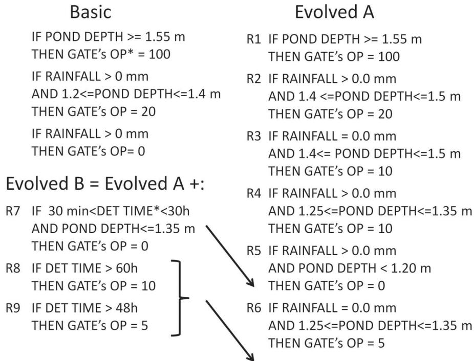
Figure 7. Rules of the first three developed RTC scenarios. OP = opening percentage; DET TIME = detention time.
