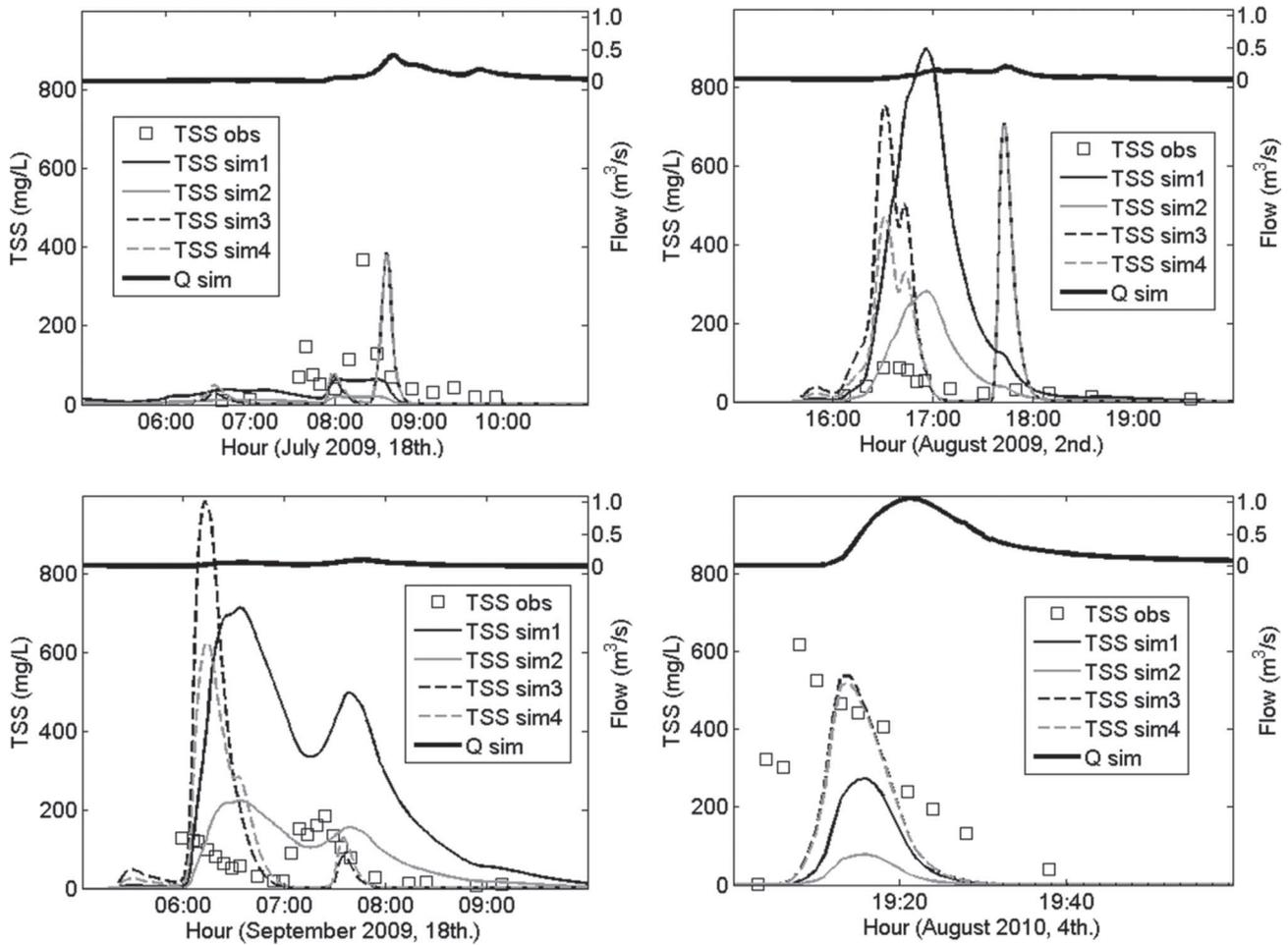
Figure 6. Observed (TSS obs) and simulated (TSS sim) TSS concentrations at the pond’s inlet (validation period). The corresponding pond’s inflow (Q sim) is represented on top of the graph. See text for details.
