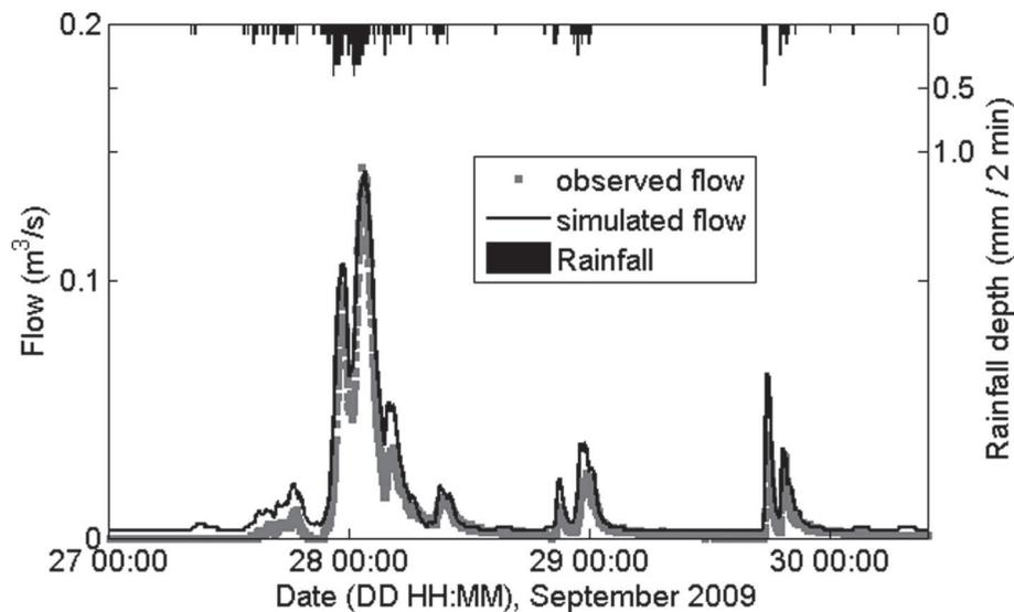
Figure 2. Observed and simulated pond's outflow with fully opened outlet (validation period).
