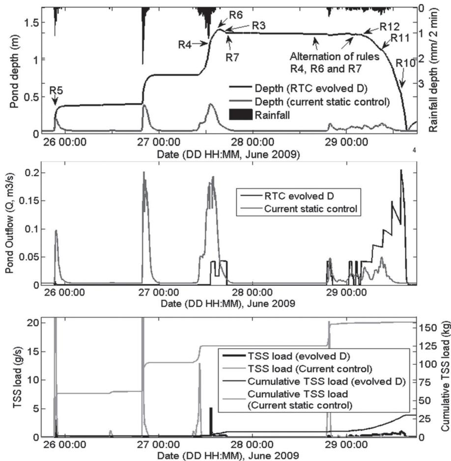
Figure 9. Example of simulated water heights (top row), outflows (middle row) and TSS discharges of the pond, with the current static control (maximum outflow limitation of  $0.35 \text{ m}^3/\text{s}$ ) and the “evolved D” RTC strategy. Explanations of the rules are given in Figures 7 and 8.
