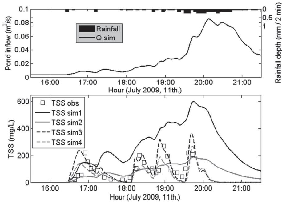
Figure 4. Observed (TSS obs) and simulated (TSS sim) TSS concentrations at the pond's inlet (calibration period). The corresponding pond's inflow (Q sim) is represented on top of the graph. See text for details.
