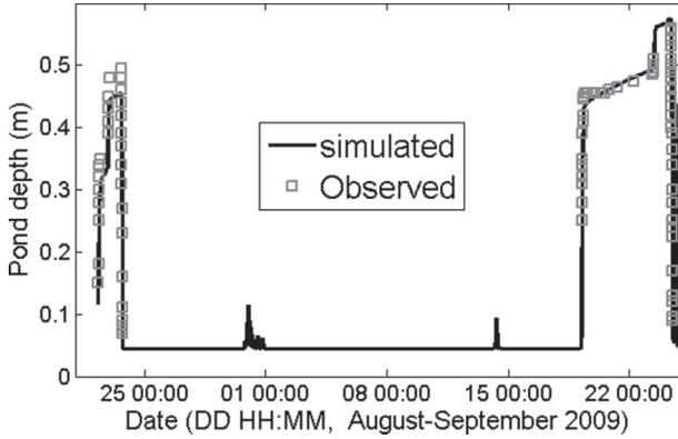
Figure 3. Observed and simulated pond's water heights during campaigns performed with the outlet closed (validation period).
