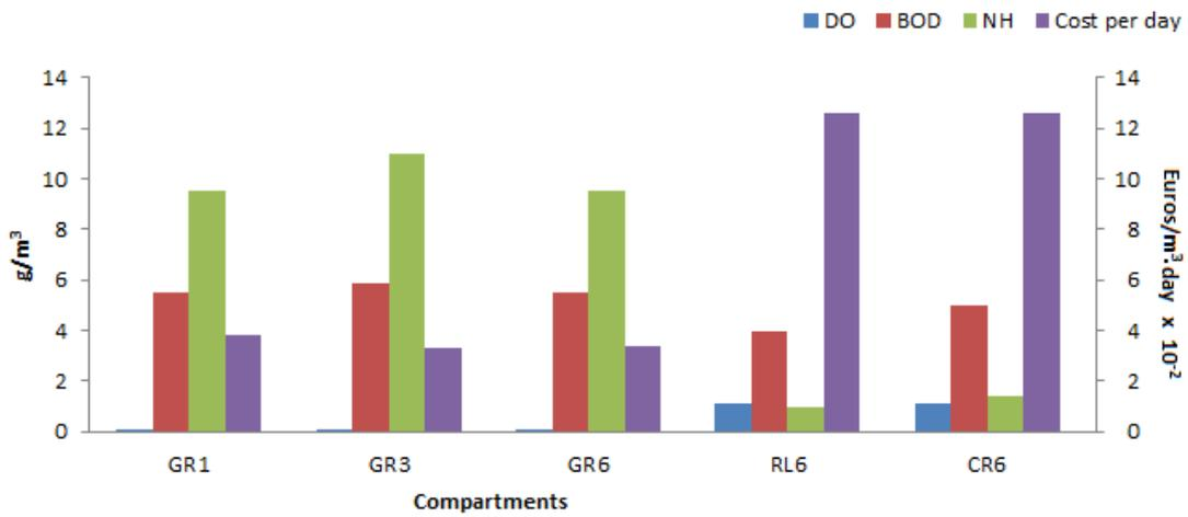
Figure 4: Effluent quality & aeration cost per day with a fixed DO setpoint of 1.5g/m<sup>3</sup>
