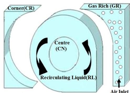
Figure 2: Cross-sectional compartments (Le Moulec et al., 2010)
