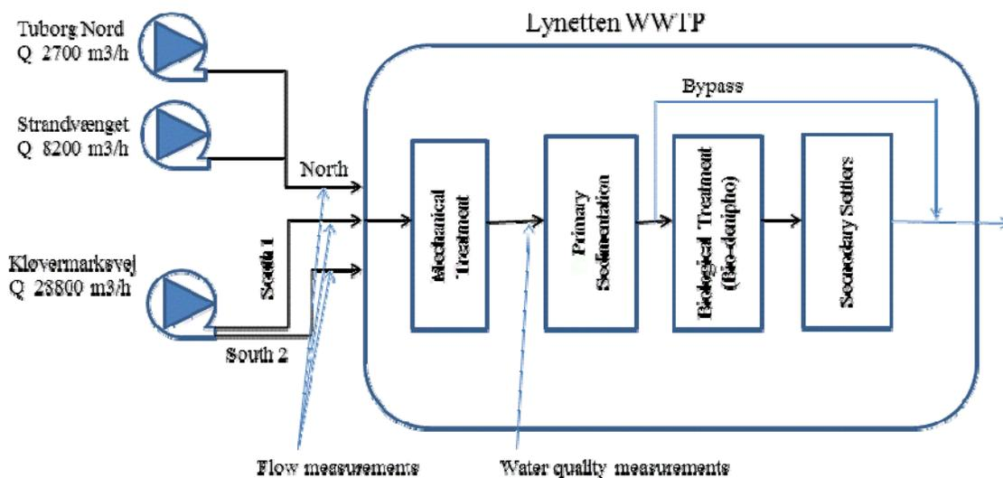
**Figure 1.** Schematic overview of pumping stations, sewer pipes, and location of the flow and water quality measurements studied in this paper.
