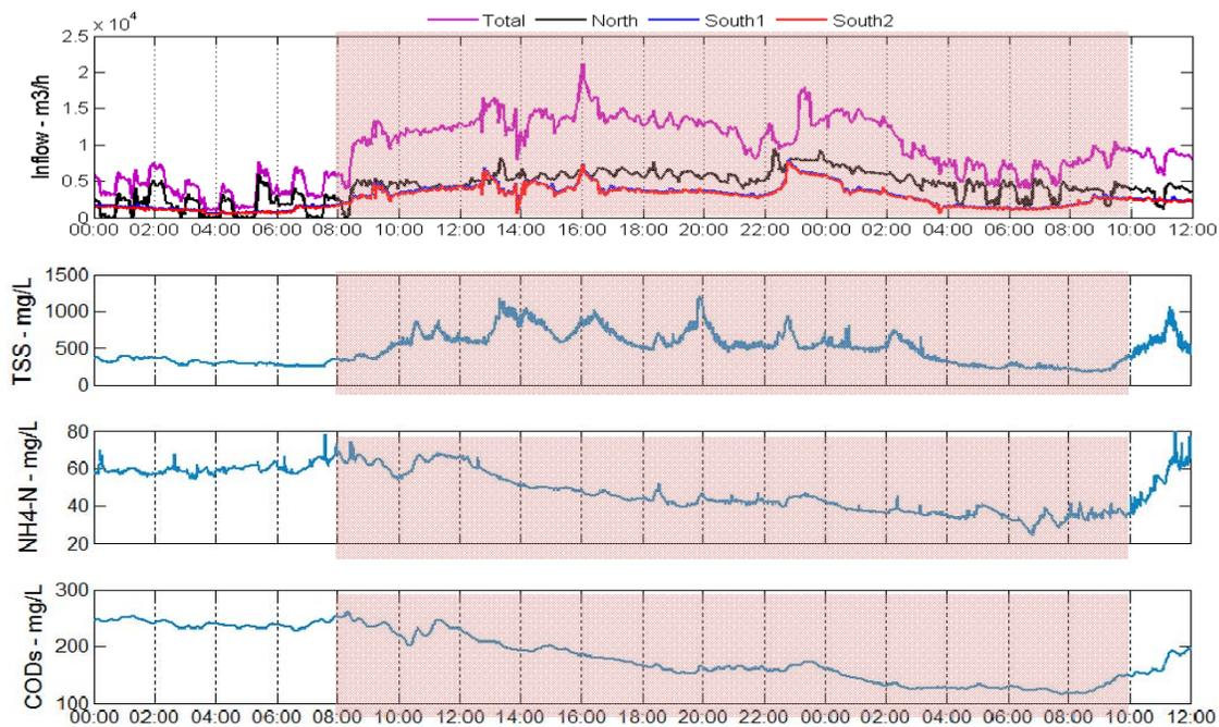
**Figure 6.** Variations in flow and water quality at the inlet of the Lynetten WWTP during wet weather (18/2 00:00 – 19/2 00:00). The marked area represents a rainfall event.
