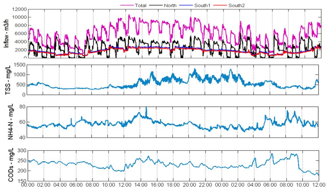
**Figure 4.** Diurnal variations in flow and water quality at the inlet of the Lynetten WWTP during dry weather (15/2 00:00 – 16/2 12:00).
