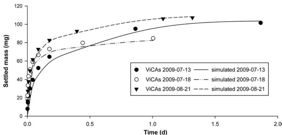
Figure 4. Results of simulations with four classes' decomposition for different ViCAs experiments. Cumulative mass observed for different ViCAs experiments compared to simulated results with the four slow classes' decomposition.
