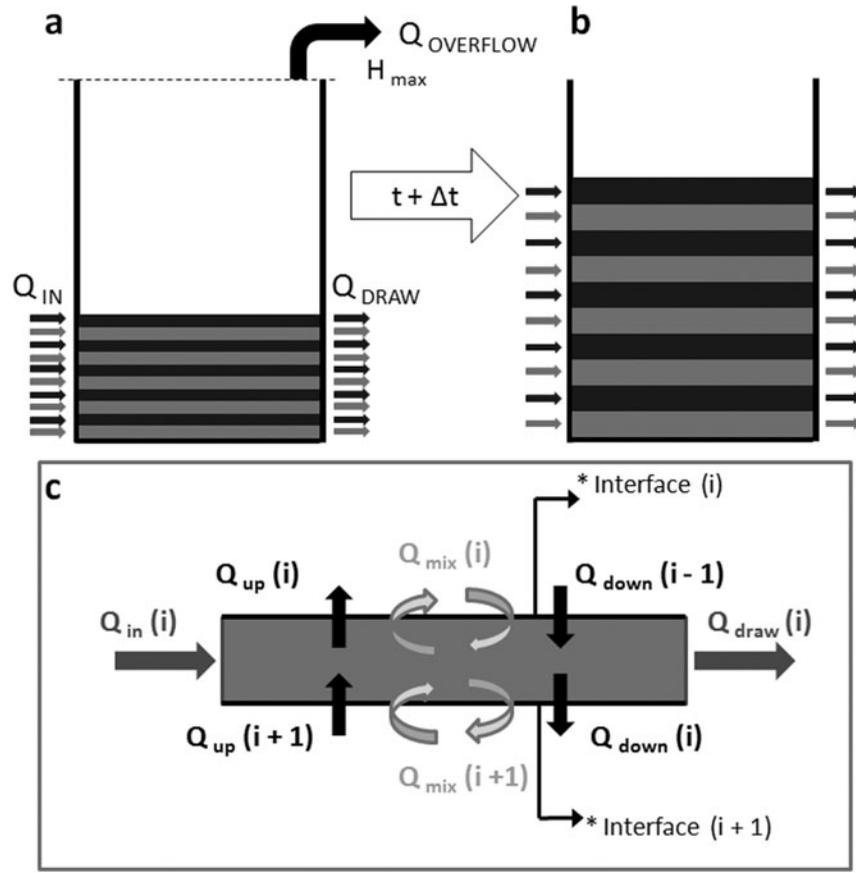
Figure 1. Hydraulic model diagram. Overview of the different variables in the hydraulic model developed. (a) and (b) present the volume change of layers in time, (c) presents the different flows accounted for in the model.
