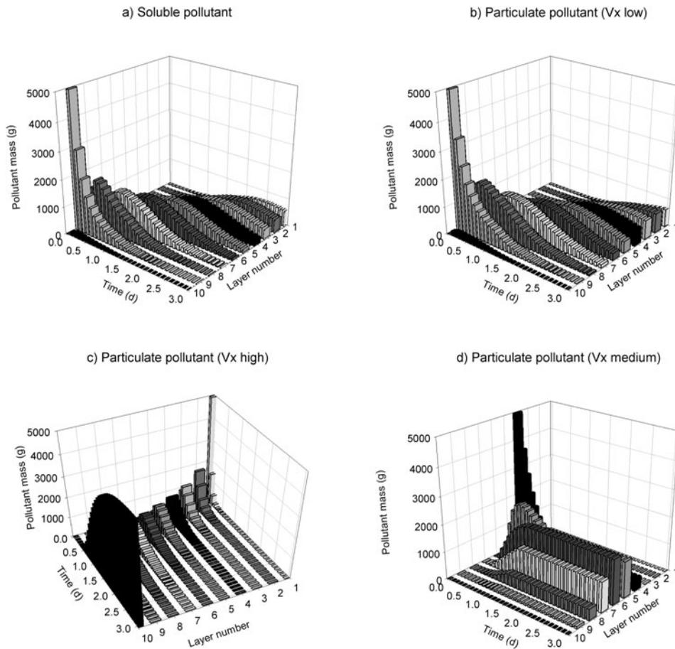
Figure 5. Dynamic pollutants' behaviour. Simulated behaviour of different types of pollutants in the developed model: Soluble pollutant (a) and particulate pollutants with low (lower than the upward water velocity) (b) high (higher than the upward water velocity) (c) and medium (equal to the upward water velocity) (d) settling velocity ( $v_x$ ).
