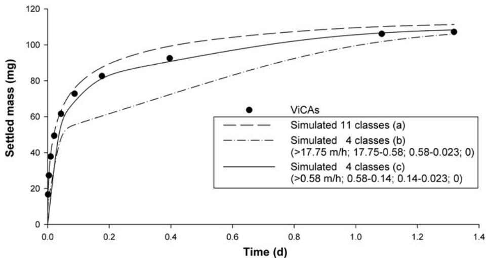
Figure 3. Results of ViCAs experiment simulations for different classes' decomposition. Cumulative mass at the bottom of a ViCAs column compared to the simulation results for different numbers (a or b, c) and types of particle classes (fast (b) or slow(c)).
