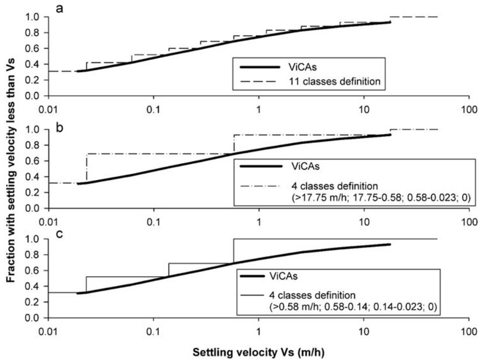
Figure 2. ViCAs experiment results and classes' decomposition. Examples of velocity classes' definition from experimental results for 11 classes (a), four classes with high settling velocities (b) and four classes with low settling velocities (c).
