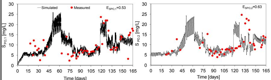
**Satisfactory results: the efficiency of the 21 model outputs range between 0.2 and 0.7 (maximum value = 1)**
