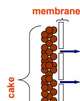
Resistances of dynamic biofilm, stable cake and pore fouling are modelled by means of in-series resistance model
