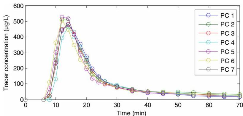
**Figure 3** | Tracer concentration profiles collected at the outlet of each of the seven parallel PCs of the Québec East WWTP. The tracer test was conducted by injecting a pulse of rhodamine WT at the inlet of each PC at  $t=0$ . The flow rate was maintained constant at about  $10,000 \text{ m}^3/\text{h}$ .
