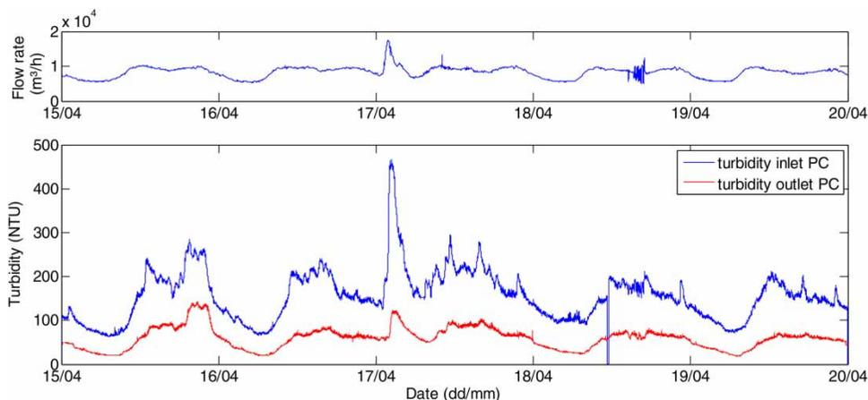
**Figure 2** | Daily dynamics of WWTP flow rate (top graph) and turbidity (bottom graph) at the inlet (top line) and at the outlet (bottom line) of the PC. On top, the WWTP influent flow rate.
