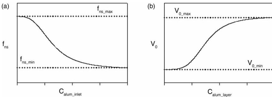
Figure 5 | Proposed evolution of (a) the non-settleable fraction of TSS,  $f_{ns}$ , and (b) settling velocity,  $V_0$ , depending on the alum concentration at the inlet of the PC and the local alum concentration in the considered layer, respectively  $C_{alum\_inlet}$  and  $C_{alum\_layer}$ .
