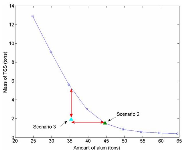
**Figure 9** | Evolution of the cumulative mass of excess TSS, i.e. when the TSS concentration is higher than the controller set-point over the 5-day evaluation period presented in Figure 7, for different constant alum concentration additions. Scenario 2 (green triangle) and 3 (blue triangle) have been highlighted. The full colour version of this figure is available in the online version of this paper, at <http://dx.doi.org/10.2166/wst.2016.600>.
