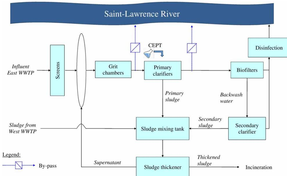
Figure 1 | Schematic process flow diagram of the Québec City East WWTP.
