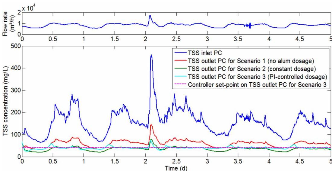
Figure 7 | PC inlet and outlet TSS concentrations for the three simulated scenarios (no alum dosage, constant dosage and PI-controlled dosage). On top, the WWTP influent flow rate.
