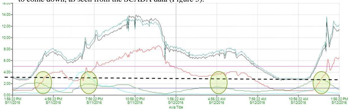
**Figure 5 – Eindhoven WRRF SCADA data: DO (red line); NH<sub>4</sub><sup>+</sup> (green line, below red line)**
