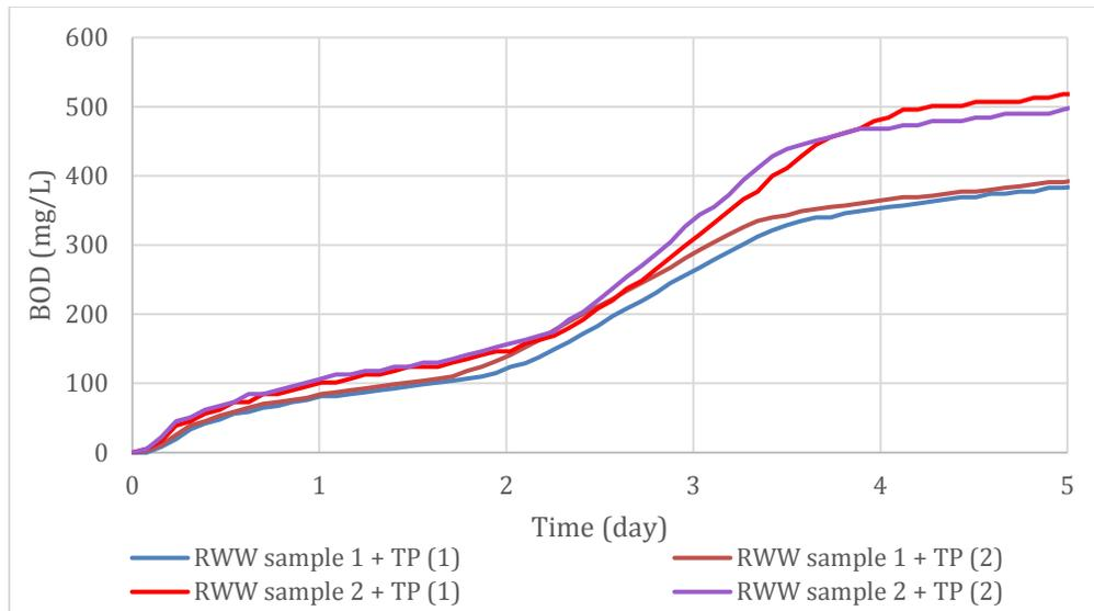
**Figure 2: 5- day BOD curves for two different wastewater samples with the addition of toilet paper (5g/l). Each experiment was performed in duplicate. All four BOD curves show a distinct increase in BOD after 2days, indicating a lag time in the degradation of toilet paper (cellulose).**
