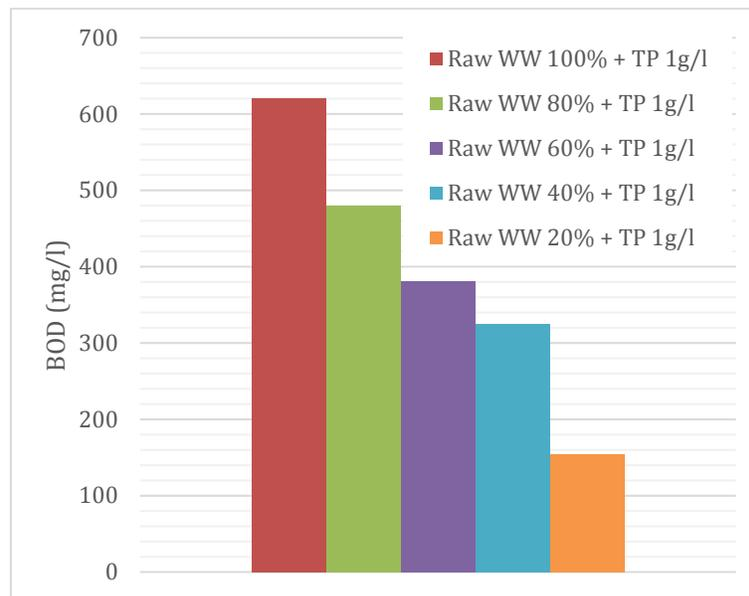
**Figure 6: BOD5 values for toilet paper in different dilutions of raw wastewater. 20% signifies a mixture of 20% wastewater and 80% tap water. The results were normalized with respect to a reference BOD curve of 100% raw wastewater to illustrate the effect of toilet paper degradation.**
