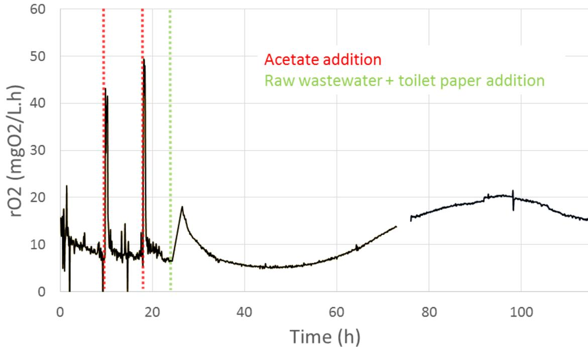
**Figure 3: Oxygen consumption rate in function of time measured in a respirometer with two additions of an acetate solution (at t=10h and t=18h, leading to initial concentration of 78 mgCOD/L) and an addition of raw WW spiked with 5g/l of toilet paper (at t=24h, leading to initial concentration of 5452 mgCOD/L).**
