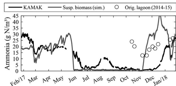
**Figure 5.** Comparison of the KAMAK™ nitrification performance with simulated performance for a suspended biomass system and the measured performance of the original lagoon without biofilm enhancement.
