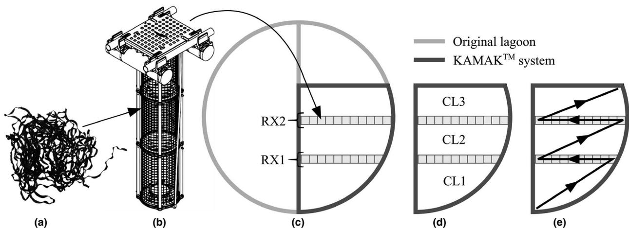
**Figure 1.** KAMAK™ system with (a) the BIONEST® media, (b) the floating columns, (c) the biofilm reactor zones RX1 and RX2, (d) the sedimentation and accumulation zones CL1, CL2, and CL3, and (e) the flow diagram.
