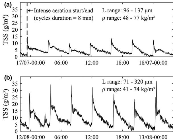
**Figure 3.** Biofilm detachment dynamics and biofilm characteristics in RX1 (a) before and (b) during the nitrification loss episode.
