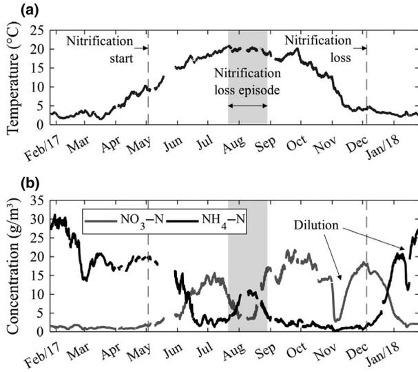
**Figure 2.** Effluent (a) temperature, (b) ammonia and nitrates over the one-year monitored period.
