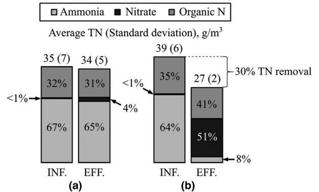
**Figure 4.** Average nitrogen fractionation for the influent and the effluent (a) during the cold period and (b) the warm period (omitting the nitrification loss episode).
