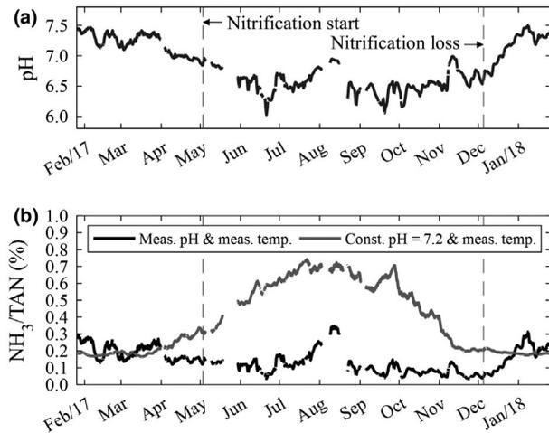
**Figure 6.** Effect of (a) effluent pH on (b) percent  $\text{NH}_3$  relative to TAN concentration.
