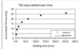
Measurement of TSS collected in cups under the hanging column of wastewater sample
