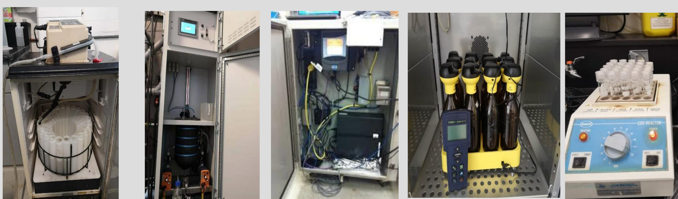
Sampling frequency: 1/hour RODTOX: Ss online monEAU station online Ultimate BOD offline Offline COD measurement
