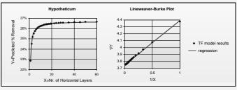
$\textbf{\textit{R}} \, \textbf{at} \sim \textbf{layers}$  (perfect plug flow) can be derived from any 2 points on the curve
