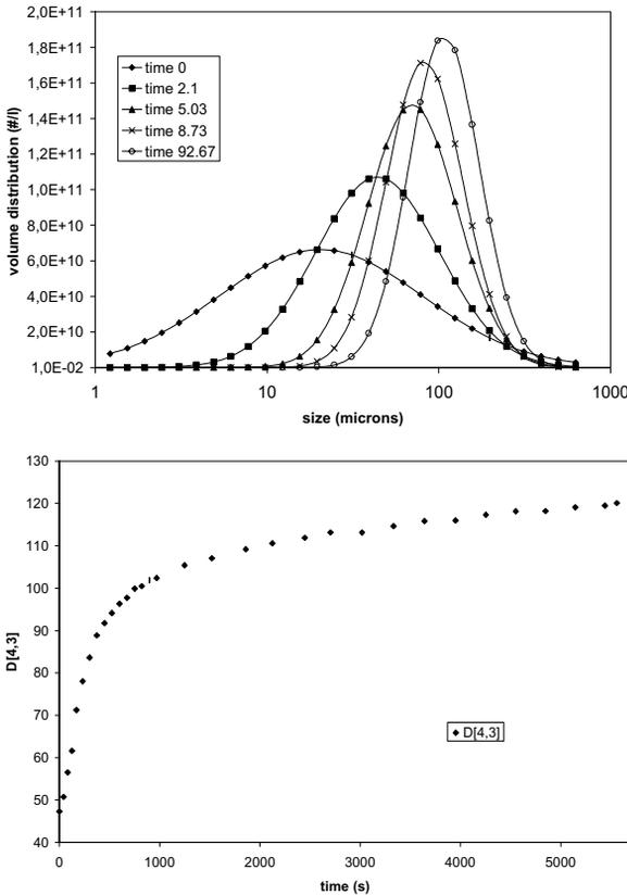
**Figure 1** Example of an on-line measurement of the dynamical change in D[4,3] due to applying a constant average velocity gradient of 37 s<sup>-1</sup>
