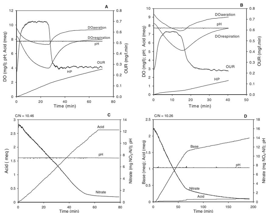
**Figure 2** Typical experimental results from the integrated sensor. The aerobic phase of the sensor: 15 ml acetate addition with pH set point 7.7 (A), 15 ml dextrose addition with pH set point 7.5 (B). The anoxic phase of the sensor: acetate addition with C/N 10.46 and pH set point 7.7 (C), dextrose addition with C/N 10.26 and pH set point 7.5 (D)
