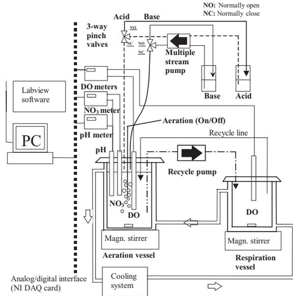
**Figure 1** Illustration of the integrated sensor set-up
