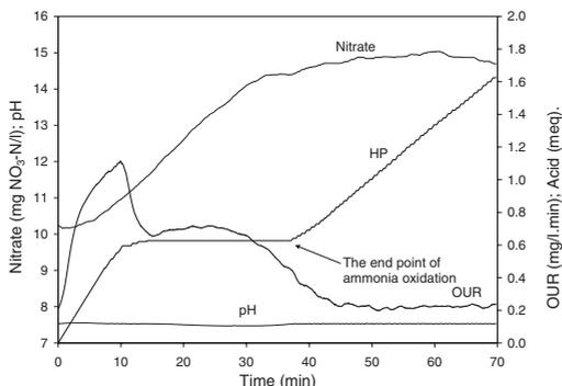
**Figure 4** Monitoring carbon source degradation and nitrification processes in single batch reactor: pulse addition of 8.5 ml acetate and 15 ml ammonium nitrogen with pH-set point 7.5
