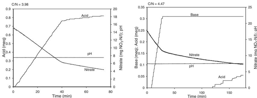
**Figure 3** Anoxic activated sludge response to low COD/N conditions: acetate addition with C/N 3.98 and pH set point 7.5 (left), dextrose addition with C/N 4.47 and pH set point 7.5 (right)
