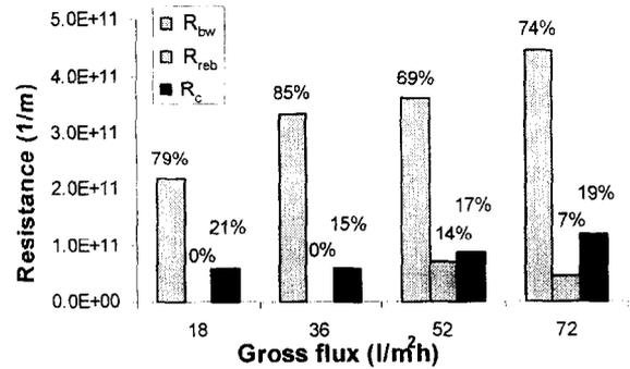
Fig. 3. Resistance due to blocking and cake as a function of gross flux.
