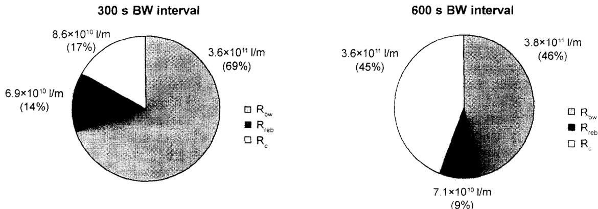
Fig. 5. Comparison blocking and cake resistance with two backwashing intervals (gross flux  $52$  l/m<sup>2</sup>h).
