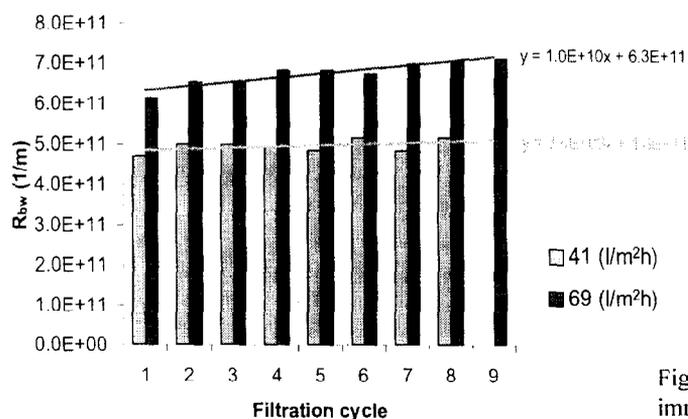
Fig. 6. Estimation of the rate of increase in initial resistance immediately after backwashing.
