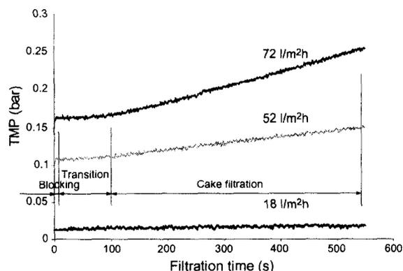
Fig. 2. Steps of membrane fouling in MBR.
