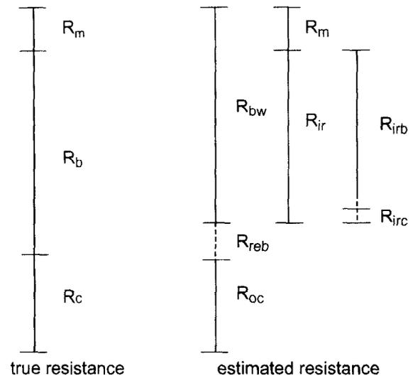
Fig. 4. Estimating blocking and cake resistance in a filtration cycle.
