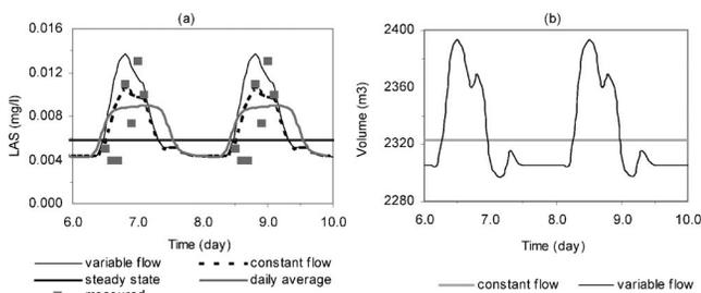
Fig. 8. Comparison of the steady-state and dynamic simulations for linear alkylbenzene sulfonates (LAS) concentration (a) and river stretch flow volume (b) in the Lambro River, Italy. In steady state, both flow and LAS concentration are assumed constant over time.
