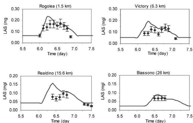
Fig. 6. Model validation results in the Lambro River, Italy. Data are simulated (lines) and measured (symbols) total linear alkylbenzene sulfonates (LAS) concentration in the bulk water.
