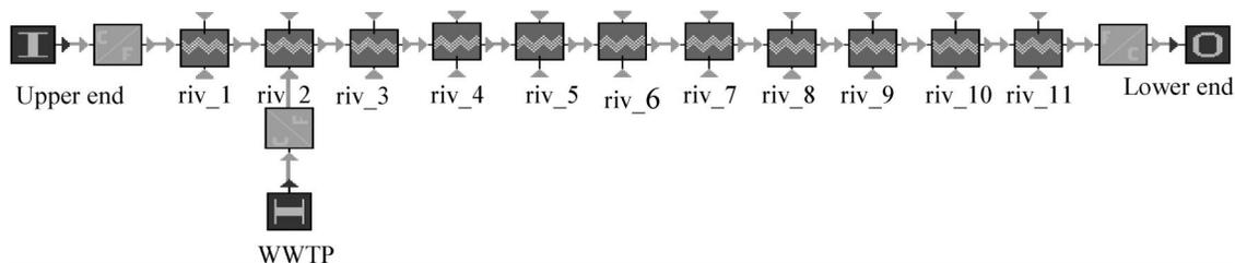
Fig. 4. Tank-in-series model for the Lambro River, Italy. Upper end is the upstream input, wastewater treatment plant (WWTP) is the side stream of wastewater discharge, and riv\_1 to riv\_11 are river reaches that are internally subdivided into a total of 47 tanks in series.
