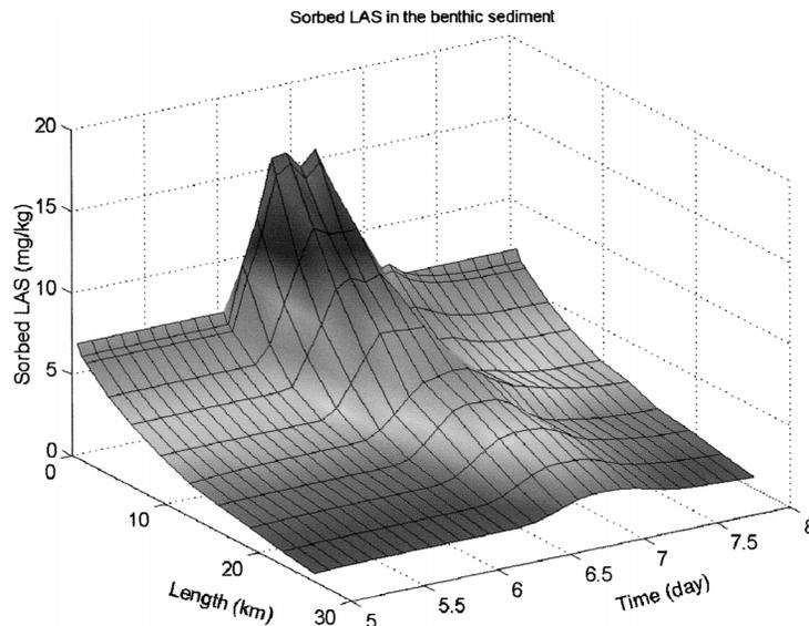
Fig. 7. Simulated sorbed linear alkylbenzene sulfonates (LAS) concentration in the benthic sediment of the Lambro River, Italy.
