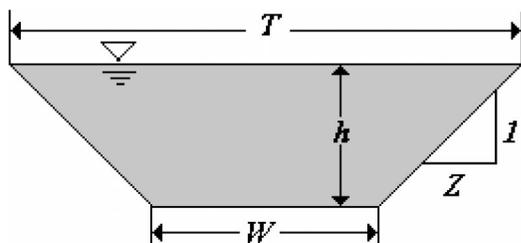
Fig. 2. Schematic representation of trapezoidal cross section for the Lambro River, Italy. Top width  $T$ , bottom width  $W$ , water depth  $h$ , and channel slope in the cross section  $1/Z$ .
