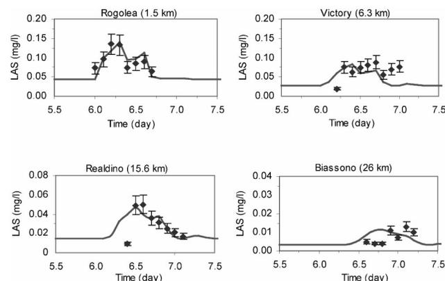
Fig. 5. Model calibration results in the Lambro River, Italy. Data are simulated (lines) and measured (symbols) total linear alkylbenzene sulfonates (LAS) concentration in the bulk water.
