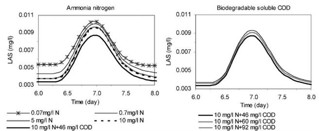
Fig. 9. The effect of nutrient dynamics on the fate of linear alkylbenzene sulfonates (LAS) in the last river section (26 km) in the Lambro River, Italy. Data are ammonia nitrogen (N) and chemical oxygen demand (COD) (as a measure of carbonaceous organic matters).
